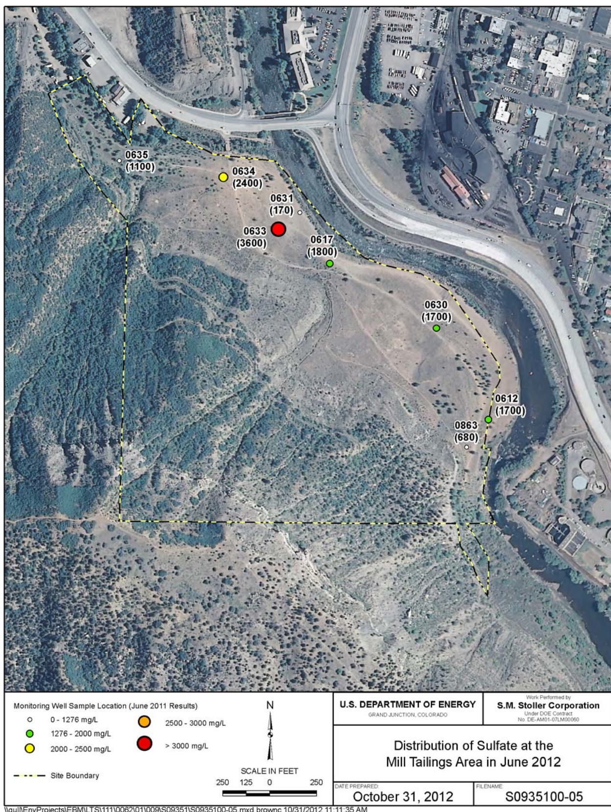
Figure 16. Distribution of Sulfate at the Mill Tailings Area in June 2012
