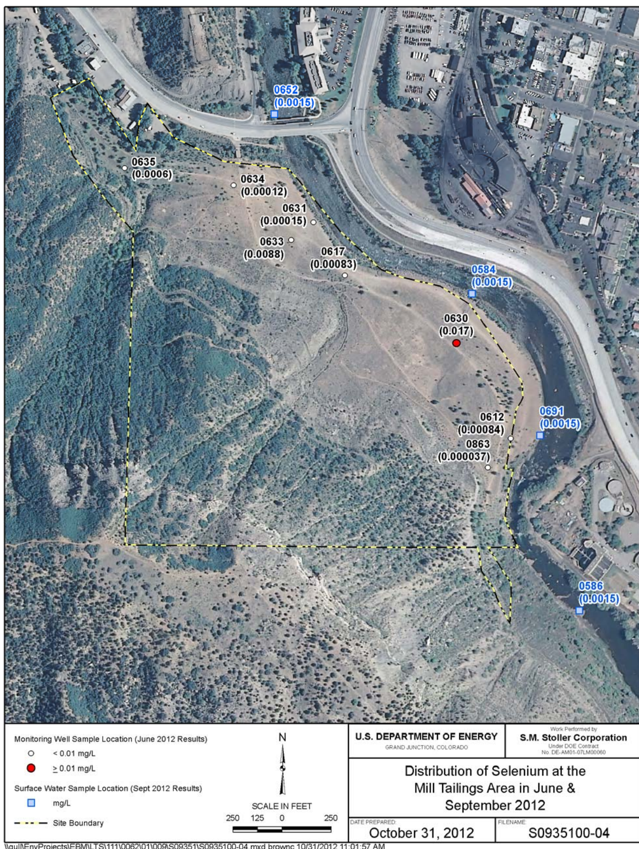
Figure 13. Distribution of Selenium at the Mill Tailings Area in June and September 2012
