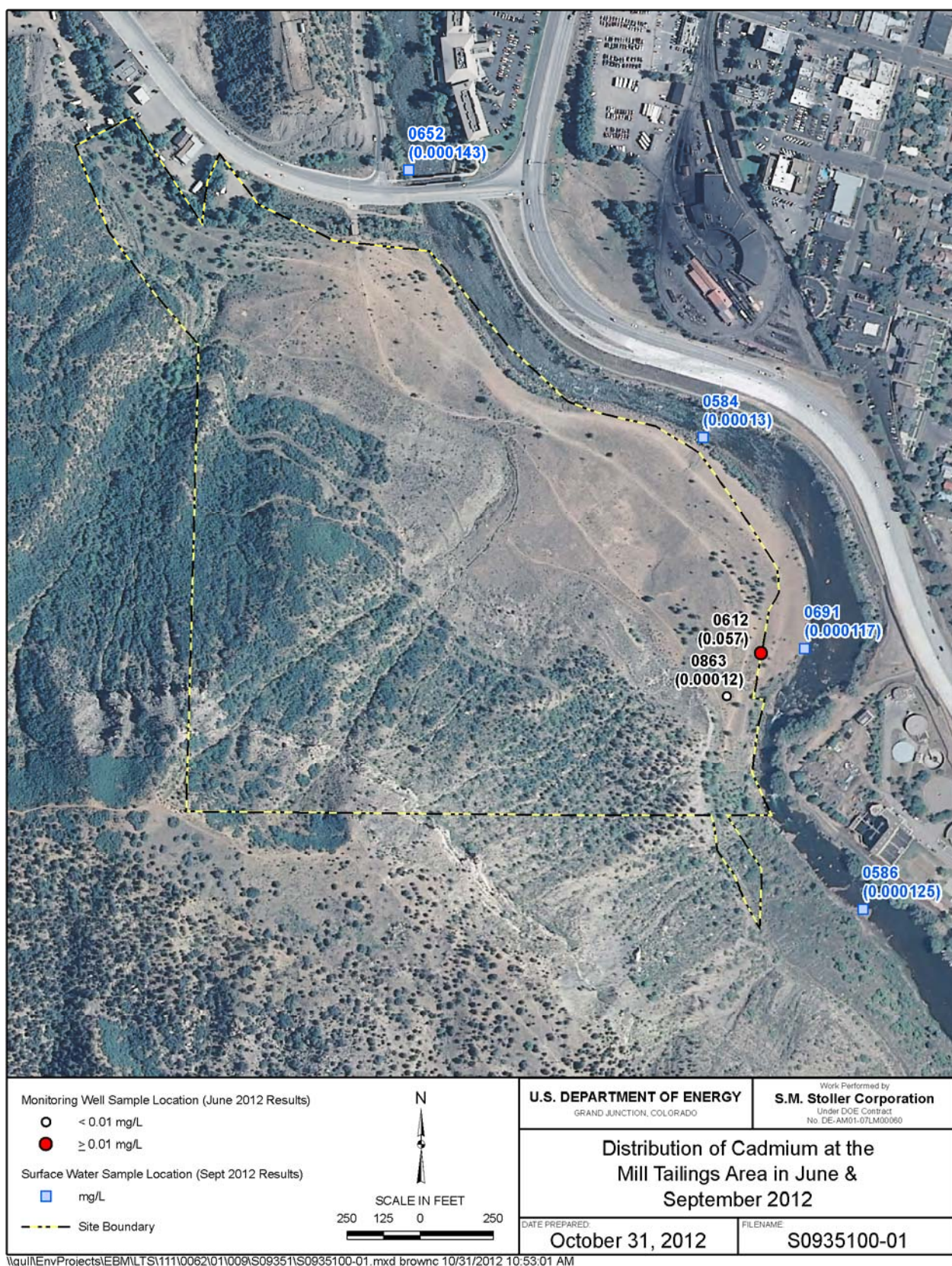
Figure 4. Distribution of Cadmium at the Mill Tailings Area in June and September 2012
