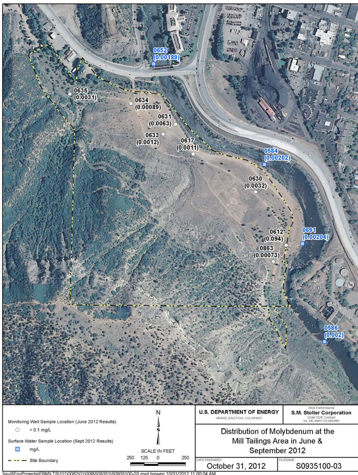
Figure 10. Distribution of Molybdenum at the Mill Tailings Area in June and September 2012
