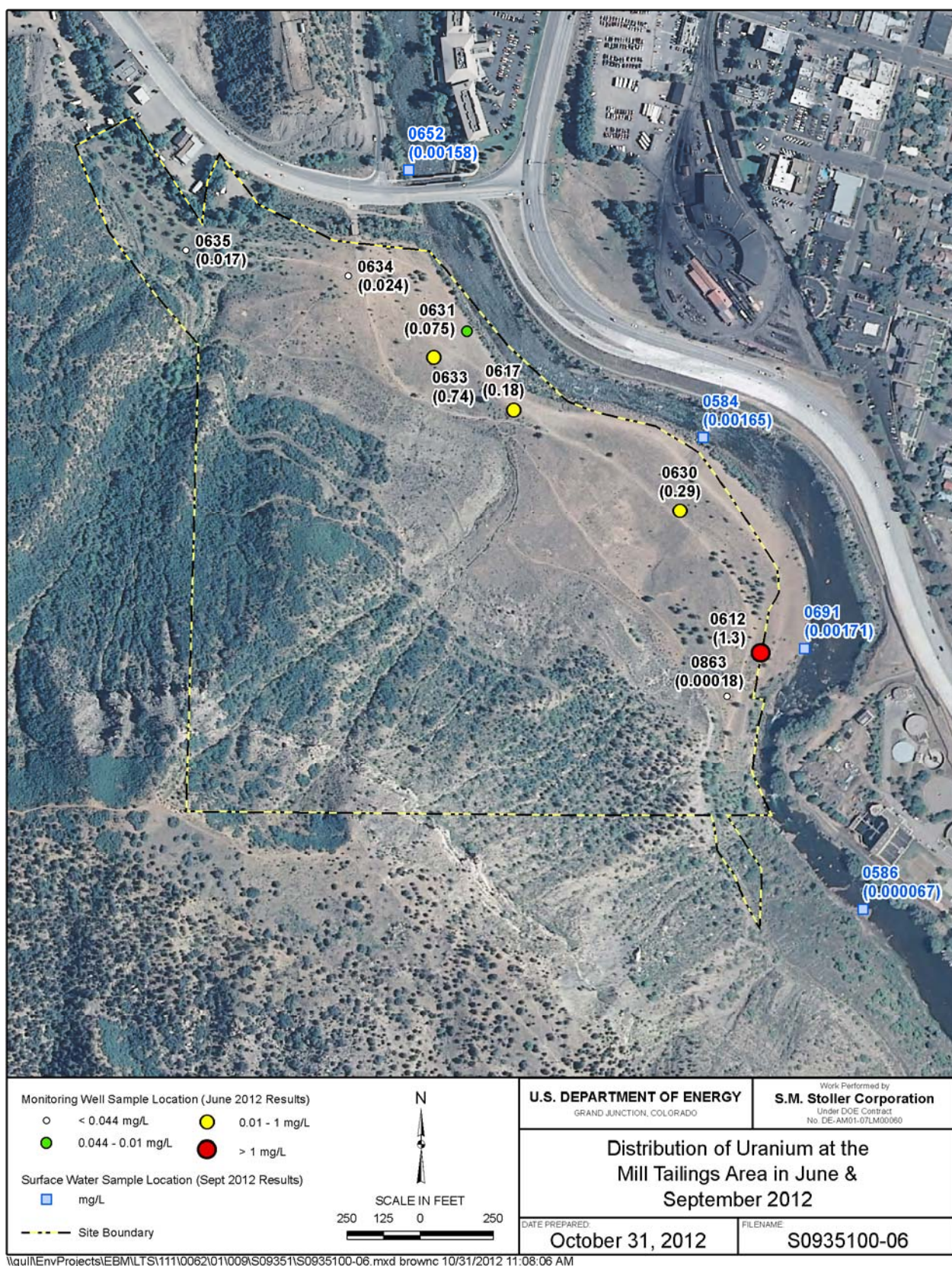
Figure 19. Distribution of Uranium at the Mill Tailings Area in June and September 2012
