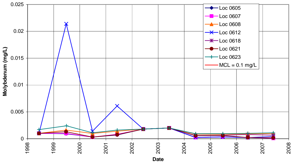
Figure 4-4. Time-Concentration Plot of Molybdenum in Groundwater at the Durango, Colorado, Disposal Site
