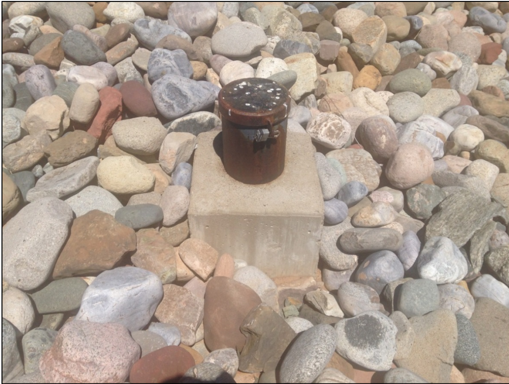
PL-9. Rocks Dug Out Around Settlement Plate 4, Likely by a Large Animal
