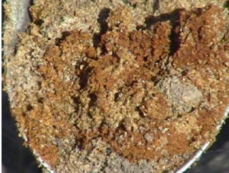
Figure 4-13. Rusty Coloration of Subpile Soils Caused by Ferric Oxyhydroxides (Location 544)
