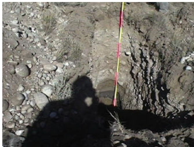
Figure 4-6. Excavation on the Millsite in November 1999 (View 2) - Note: the select fill appears as a distinct layer in the test pits
