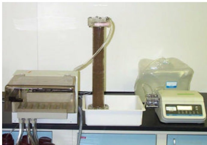
Figure 4-9. Setup of Column Experiment Note: source tank and peristaltic pump (right), column filled with subpile soil (middle) fraction collector (left)
