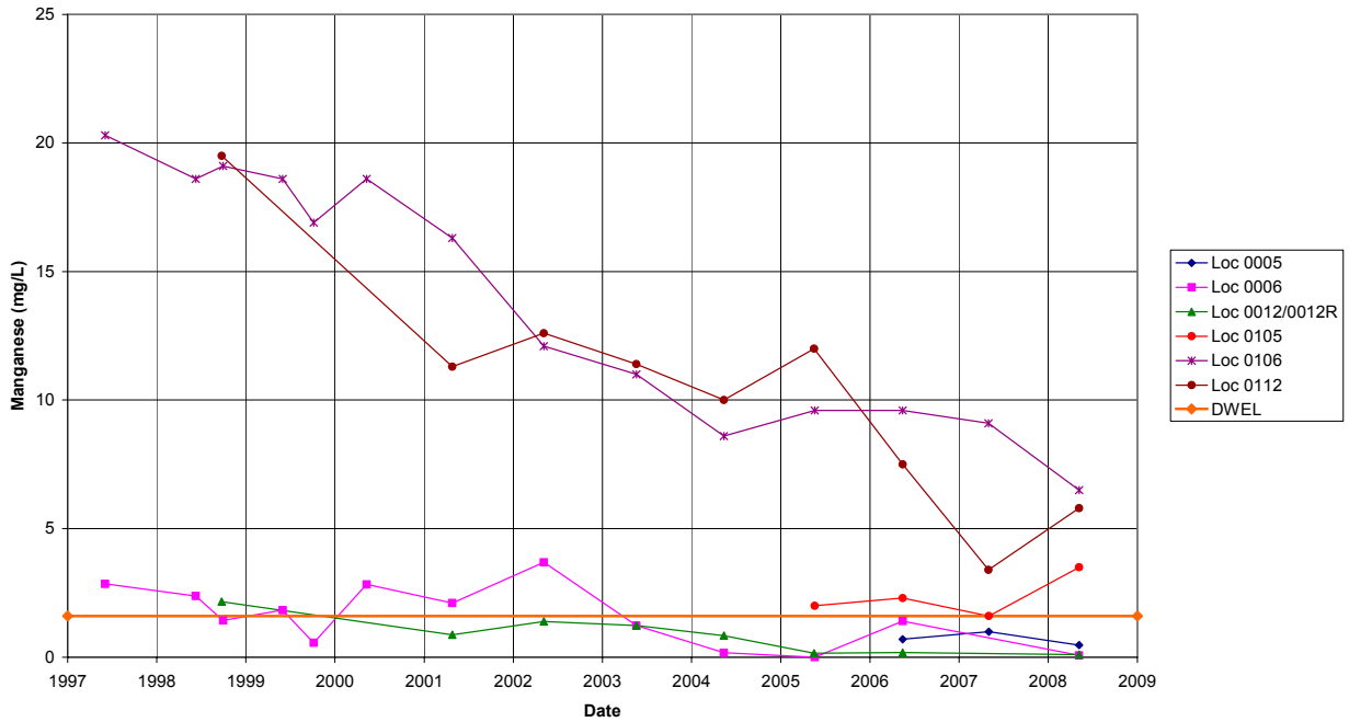
Figure 9. Manganese Concentrations in Groundwater – On-Site DOE Monitor Wells at the Gunnison Site
