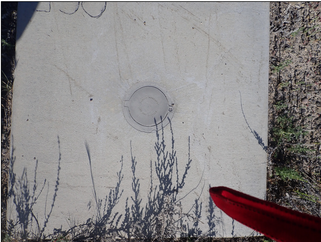
PL-2. Aerial Survey Quality Control Monument QC-5
