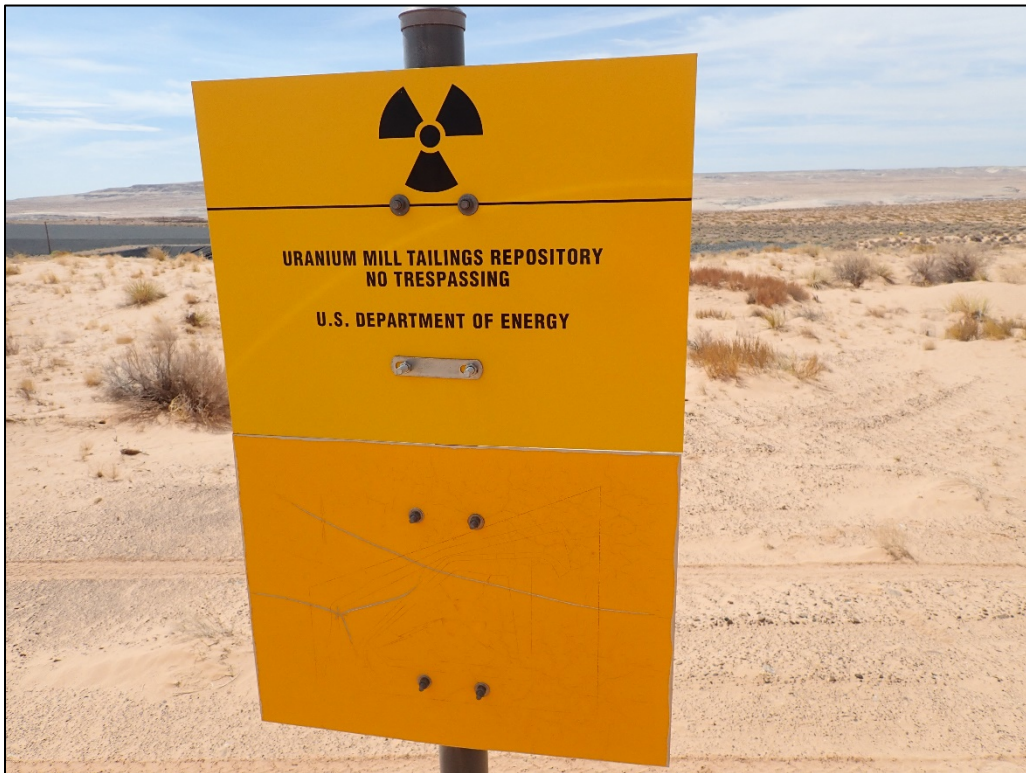
PL-2. Faded and Cracked Pictorial Perimeter Sign P6
