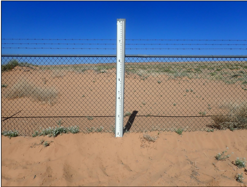
PL-3. Sediment Deposition Gage Between Perimeter Signs P9 and P10
