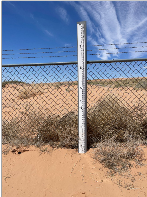
PL-3. Sediment Deposition Gauge Between Perimeter Signs P9 and P10
