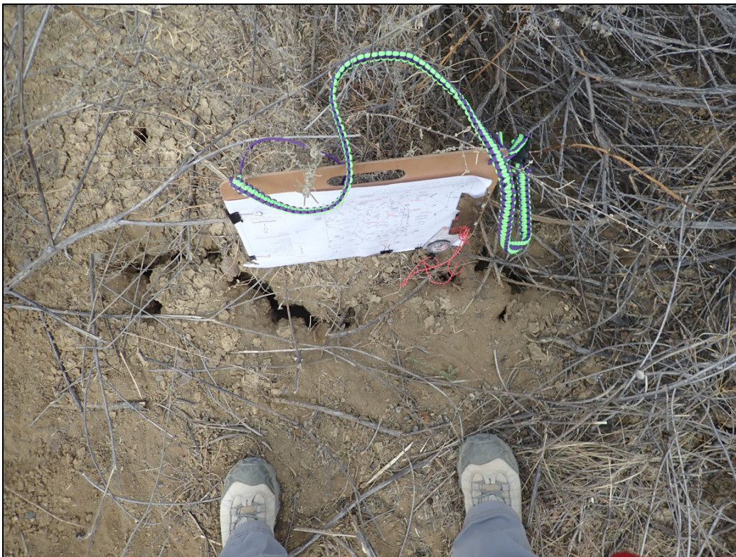
PL-12. Deep Desiccation Cracking of Surface Soils
