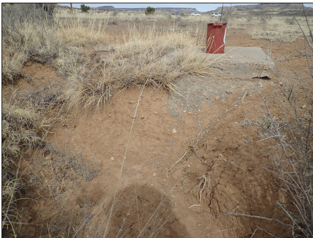
PL-8. Erosive Channeling Around Monitoring Well 62
