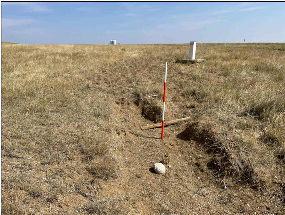
PL-8. Erosion Caused from Overflowing Water Storage Tank
