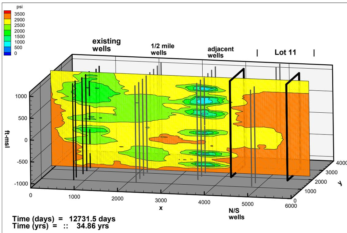
Figure 11. Simulated pressure distribution in 2045 after simulating the producing life of staged approach wells west, south, and north of the site within the 0.5-mile radius
