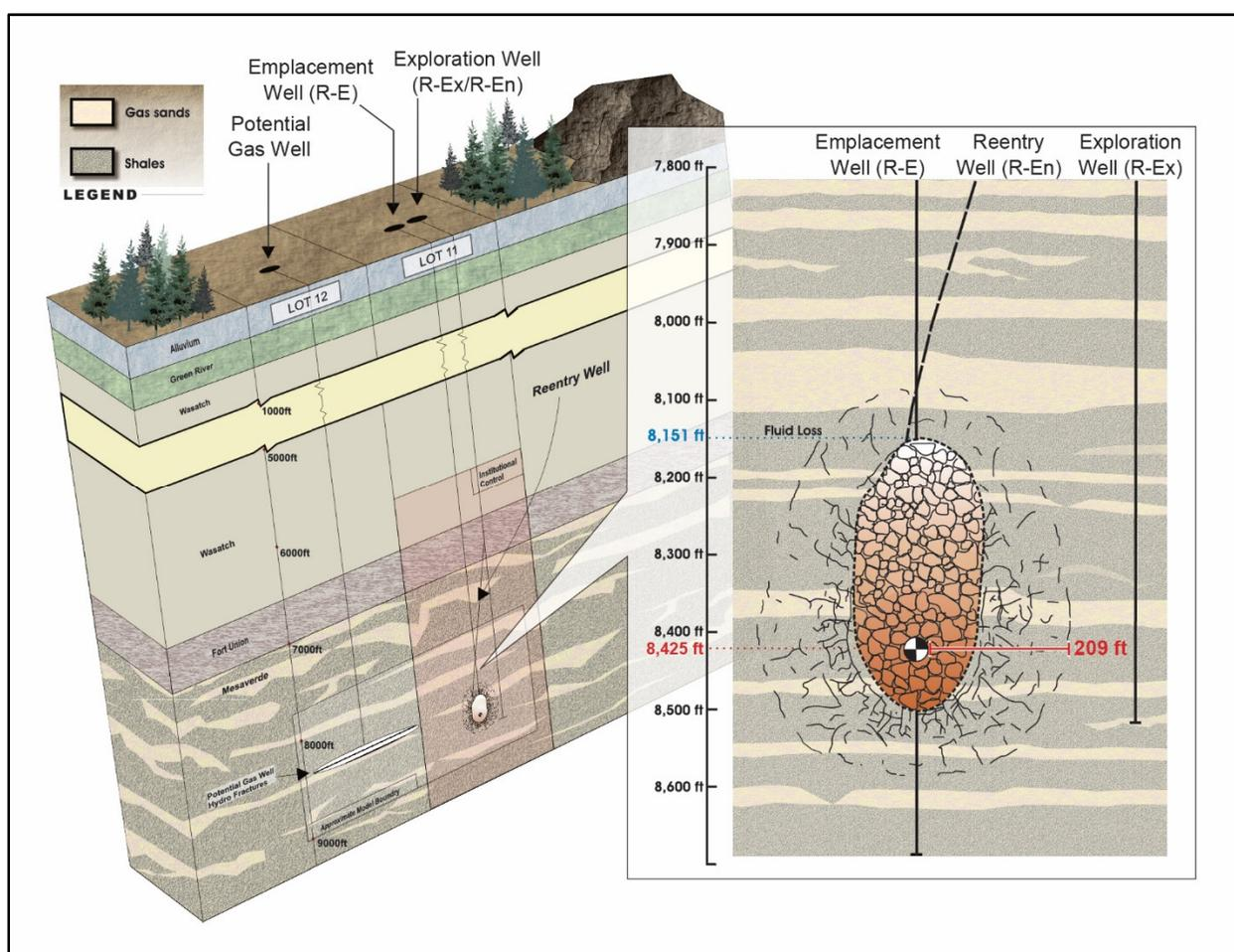
Figure 4. Schematic cross section of the Rulison site detonation zone
