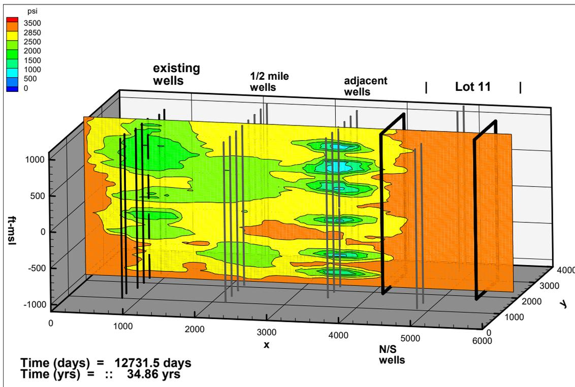
Figure 12. Simulated pressure distribution in 2045 with 2900 psi contour changed to 2850 psi
