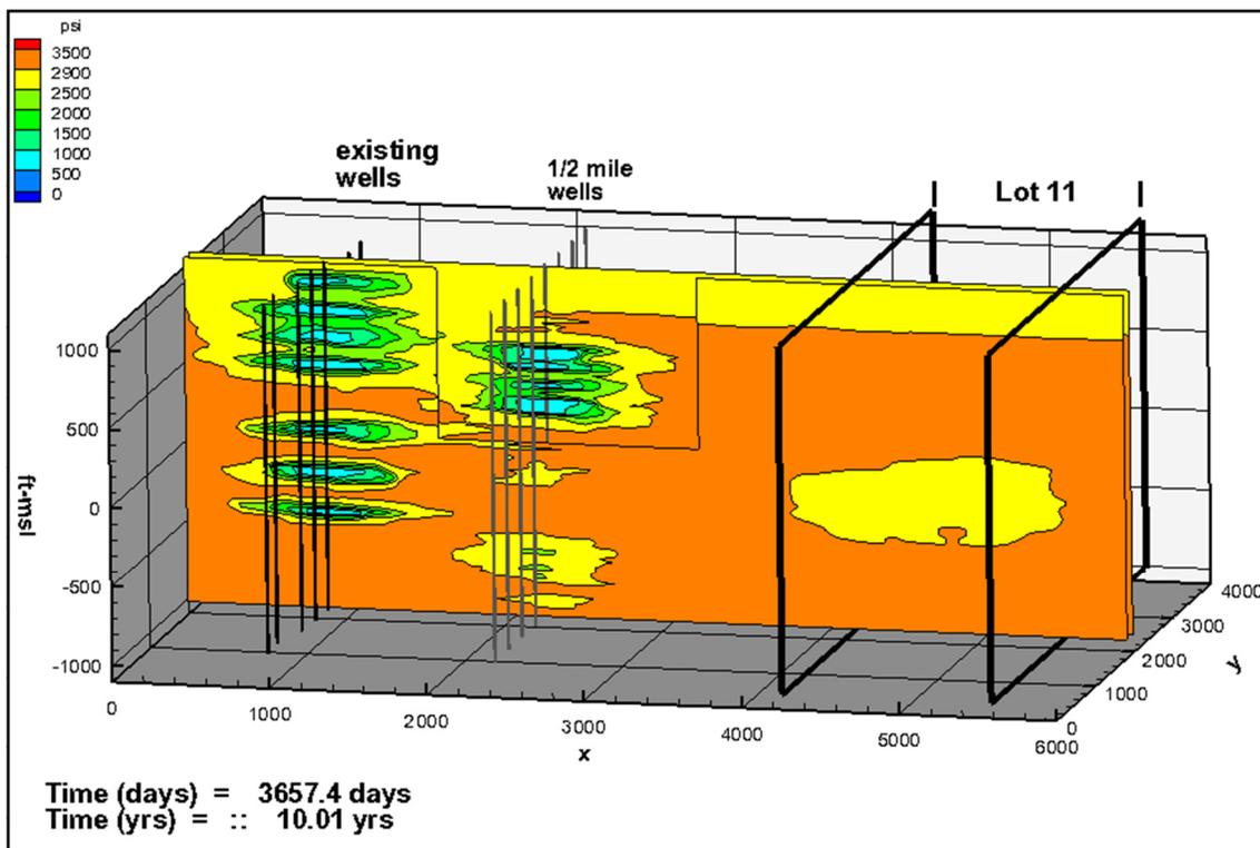
Figure 10. Simulated pressure distribution after 10 years of production from existing wells 0.75 mile and 5 years of production from potential path forward wells 0.5 mile from the detonation (year 2020)
