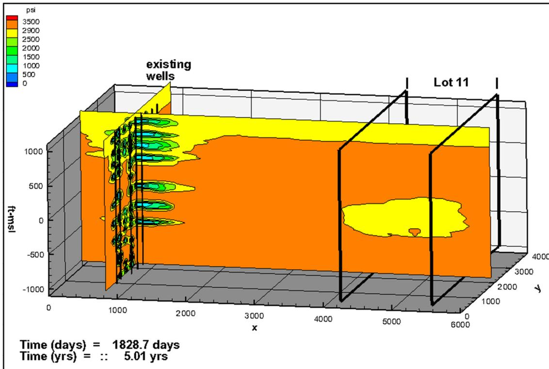
Figure 9. Simulated pressure distribution after 5 years of production from the existing active wells 0.75 mile from the detonation (year 2015)
