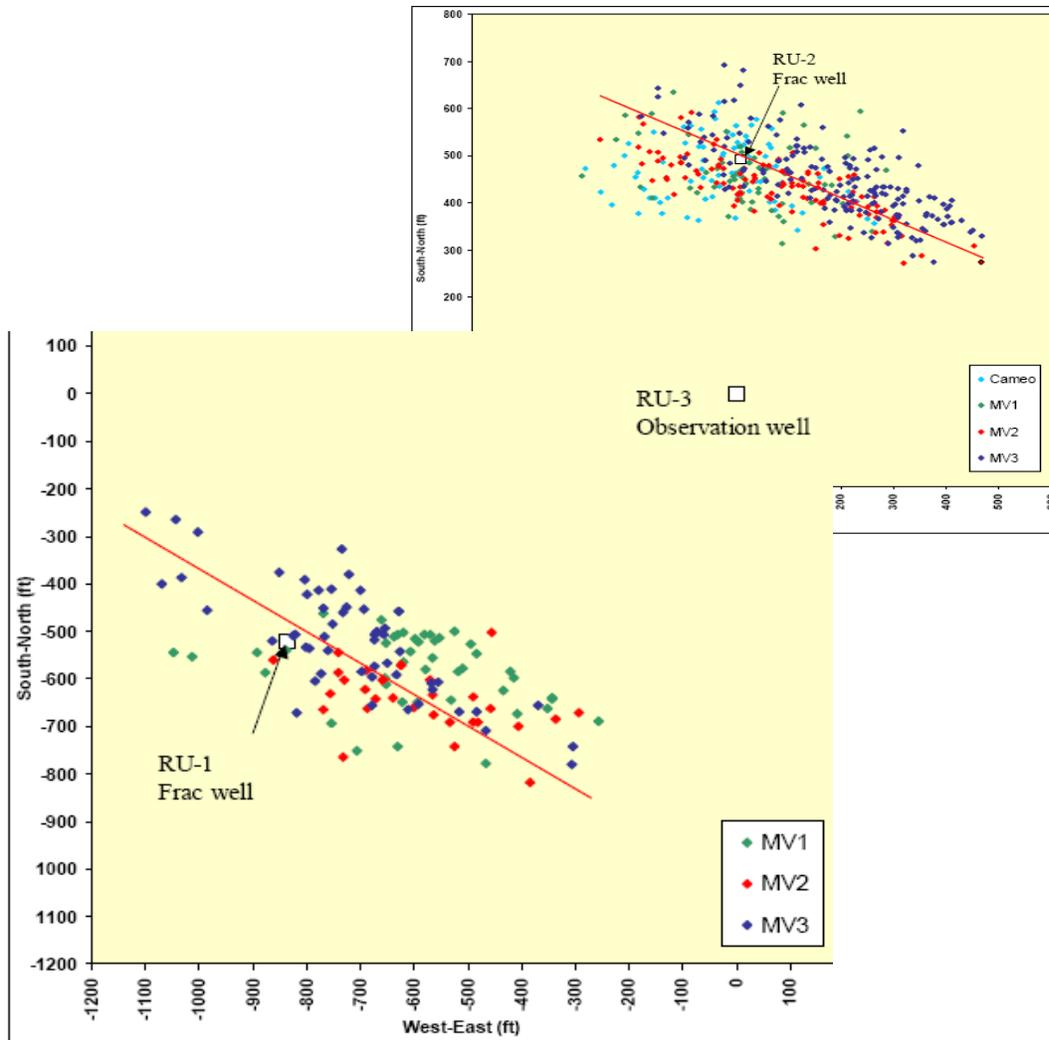
Figure 15. Microseismic mapping of the hydrofracturing of two wells
