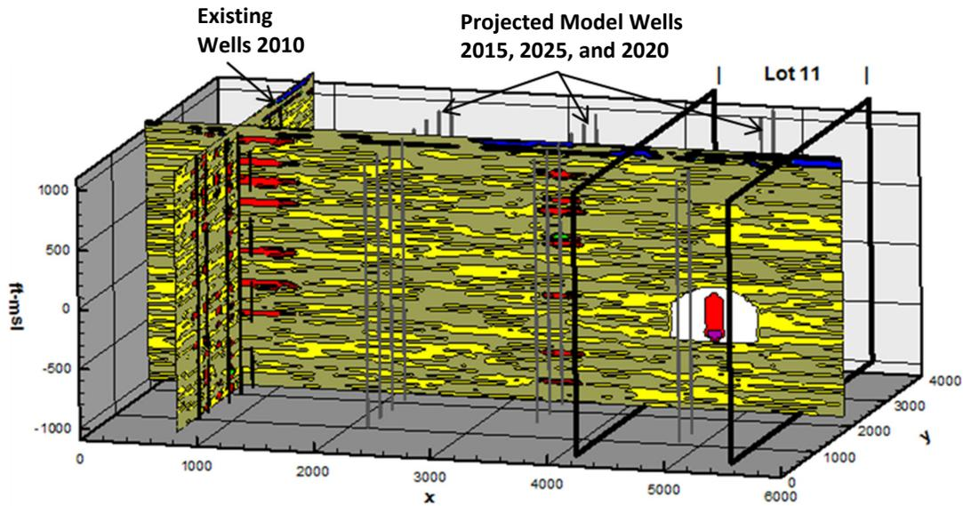
Figure 7. Fence diagram of the model domain showing the distribution of rock types yellow (lower Williams Fork sandstone gas reservoirs), olive (shale), white (nuclear fractures), red (hydrofractured sandstone, chimney), blue (upper Williams Fork sandstone), green (hydrofractured shale)
