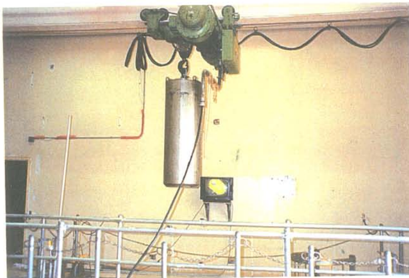
Fig. G-6. Hoist of NAC ITS Inner Shield over Dry Pit in Bldg. 21, Rm. 21/111, 9/17/03
