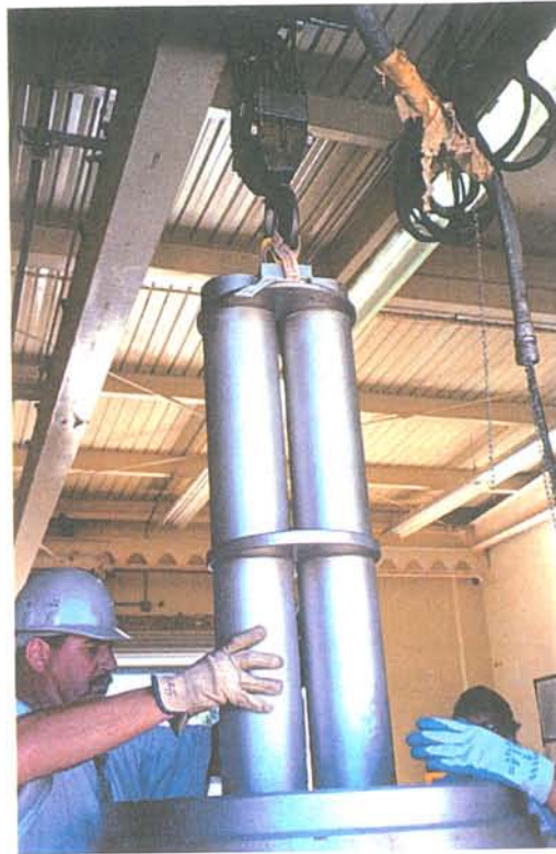
Fig. G-5. IFM Basket (NAC Top Module) Insertion into Interim Transfer System (ITS), 9/17/03
