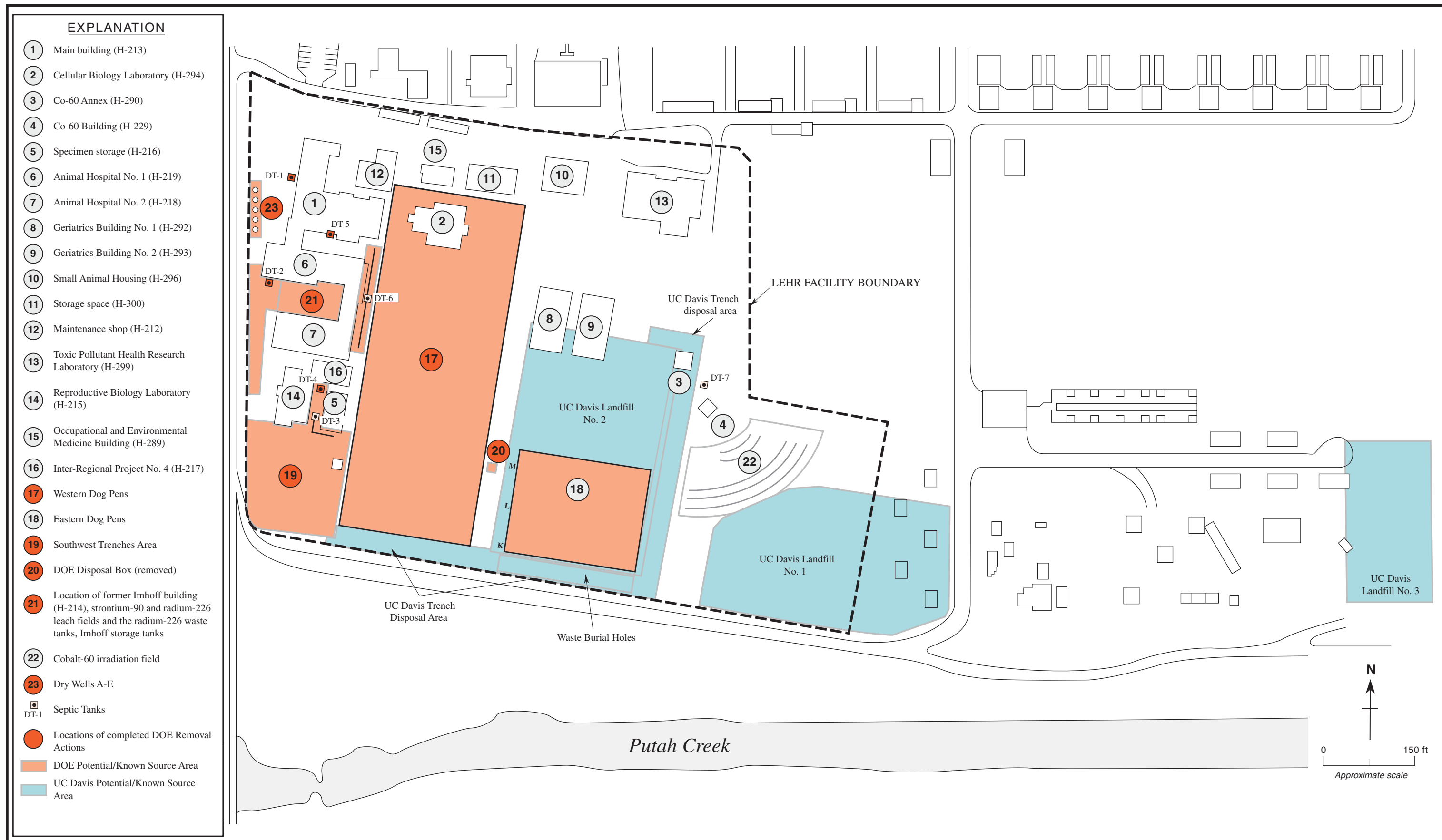
Figure 1-2. Site Features and Potential Contaminant Source Areas
