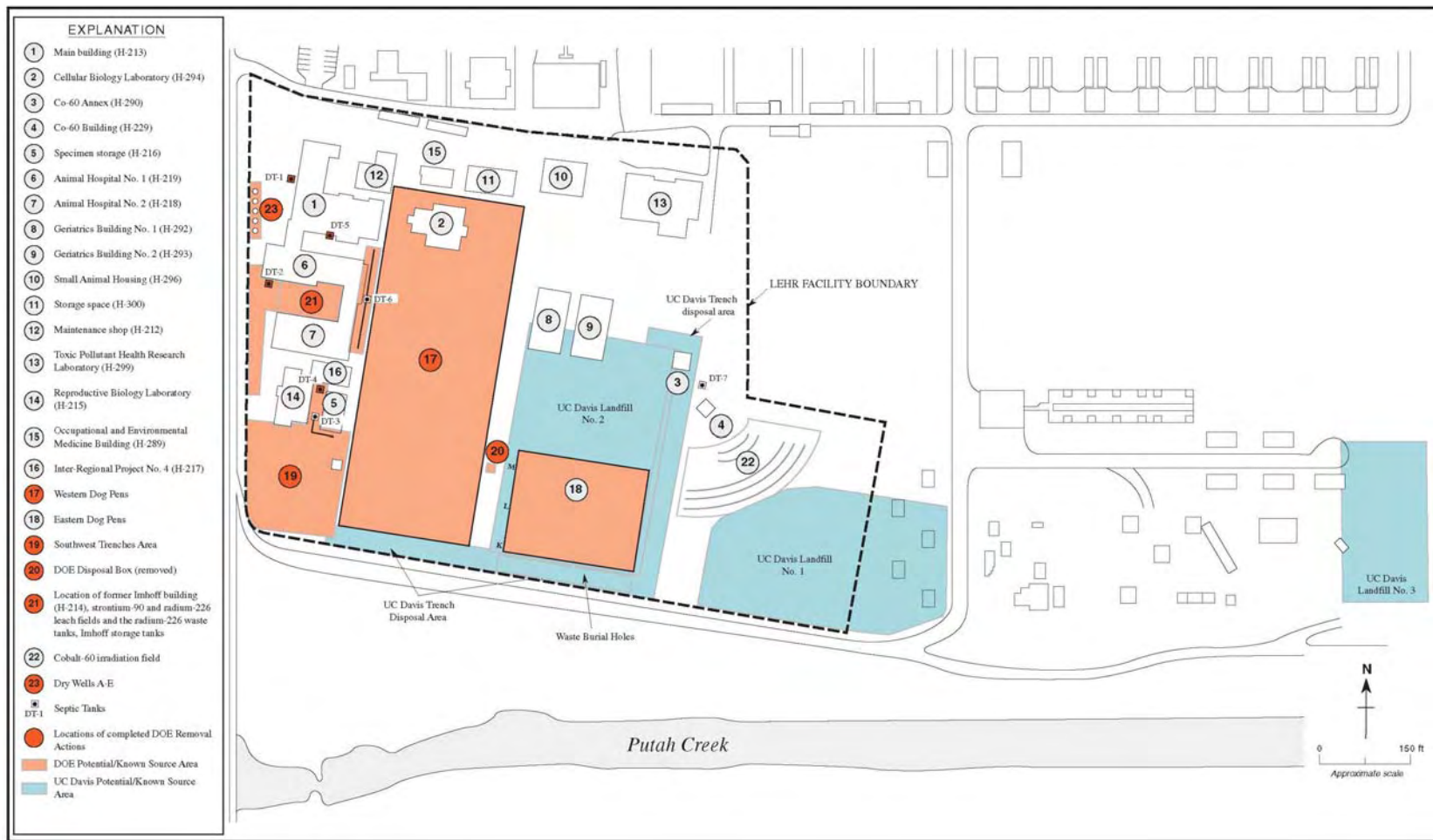
Figure 1-2. Site Features and Potential Contaminant Source Areas
