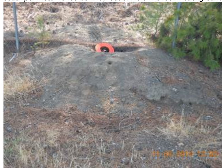
View south: Monument 18, within orange ring; foot of North Levee in background; burrow mound in foreground.
