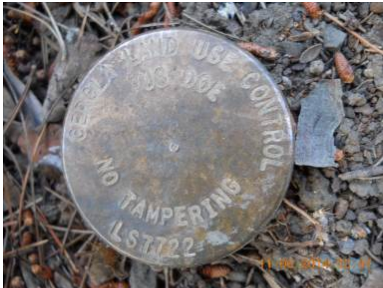
Monument 8: southwest corner of radium-226 leach trench; Radium/Strontium Treatment Systems Area.
