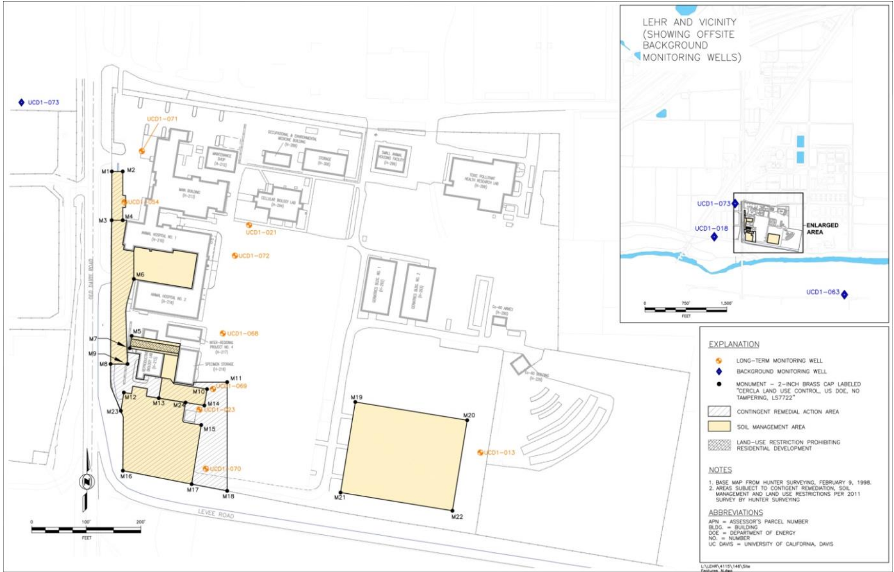
Figure 3. Monitoring Wells and Corner Point Monuments at the LEHR Superfund Site
