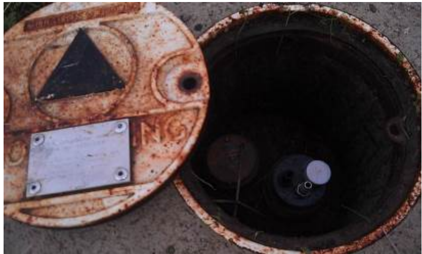
UCD1-069: new silicone stopper in water level measurement port.
