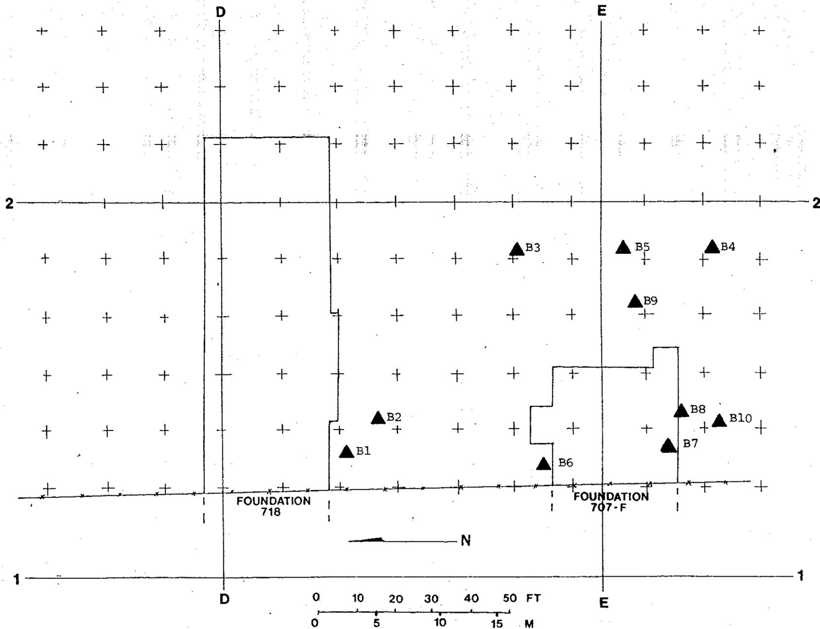
FIGURE 11. Locations of Elevated Surface Contact Radiation Levels Identified in the Vicinity of the Building Foundations. (These elevated areas were identified following the remedial action but prior to additional soil removal performed during the survey.)
