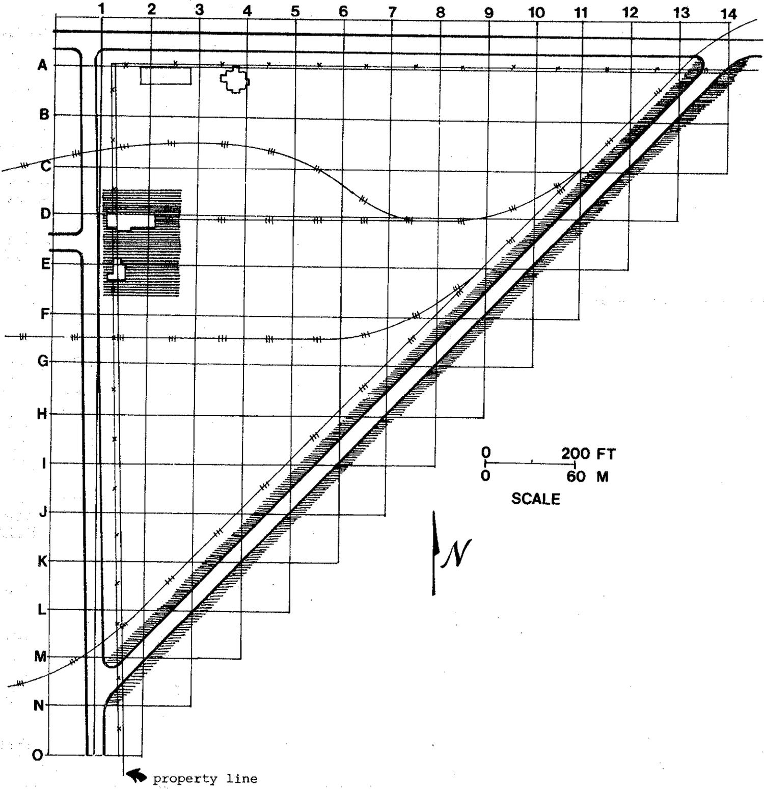
FIGURE 3. Grid System Established for Survey Reference: Shaded Regions Indicate Areas of Remedial Action.
