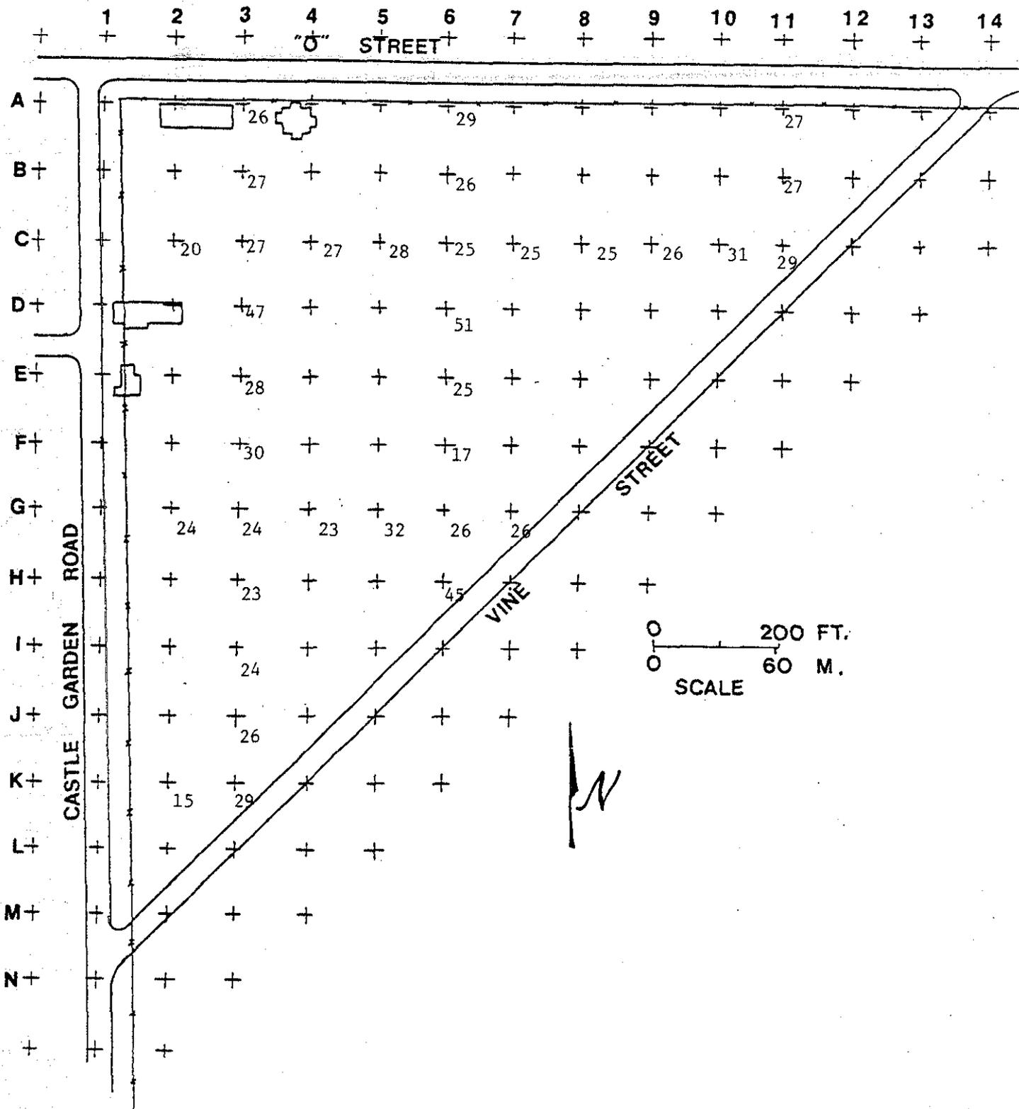
FIGURE 10. Surface Beta-Gamma Dose Rates ( $\mu\text{rad/h}$ ) Along Grid Lines C, G, K, 3, 6, and 11: Measurements to Confirm Results of the January 1971 Survey.
