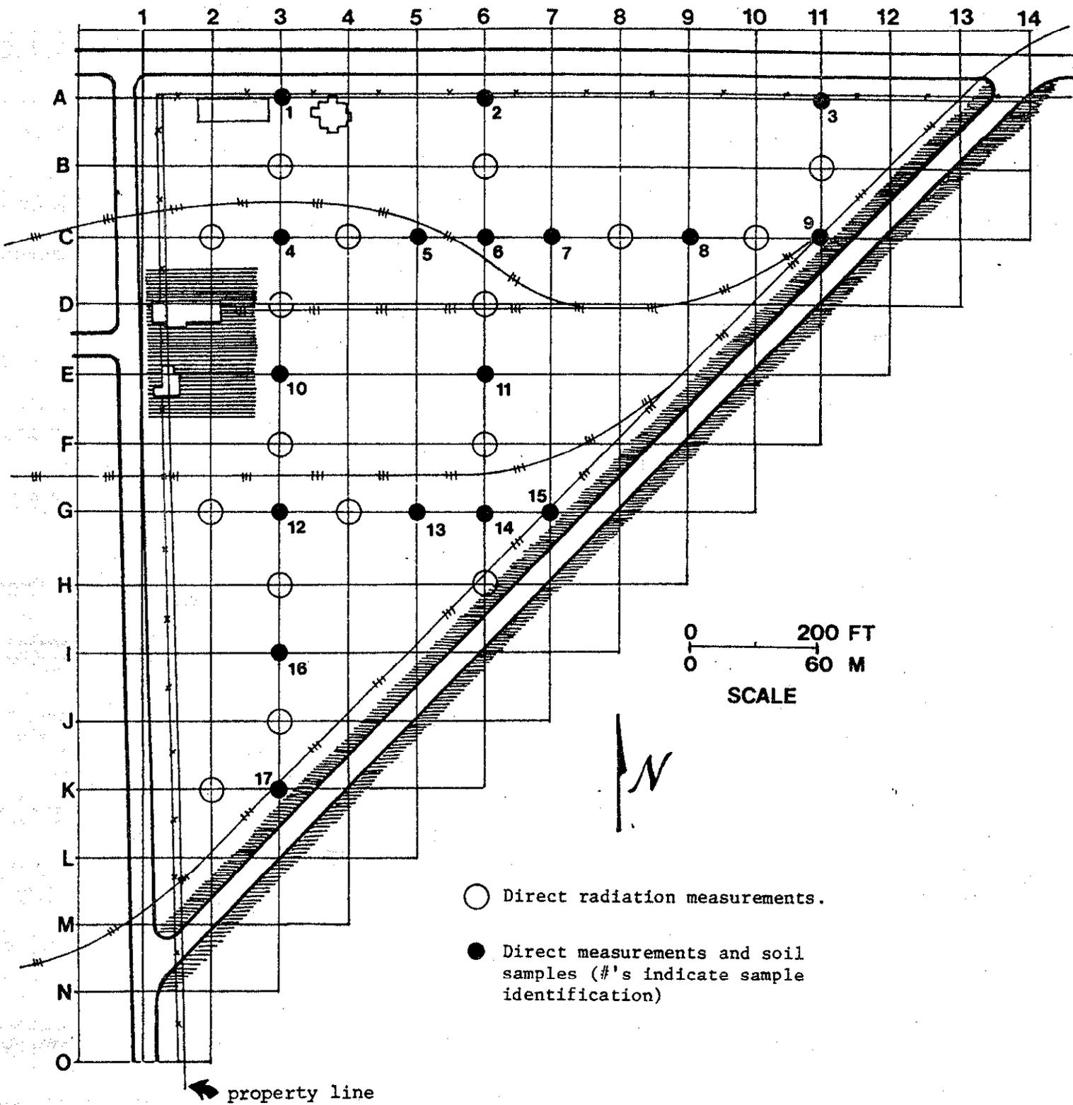
FIGURE 6. Locations of Measurements and Samples to Confirm Previous Survey Results in Areas Undisturbed by Remedial Action.
