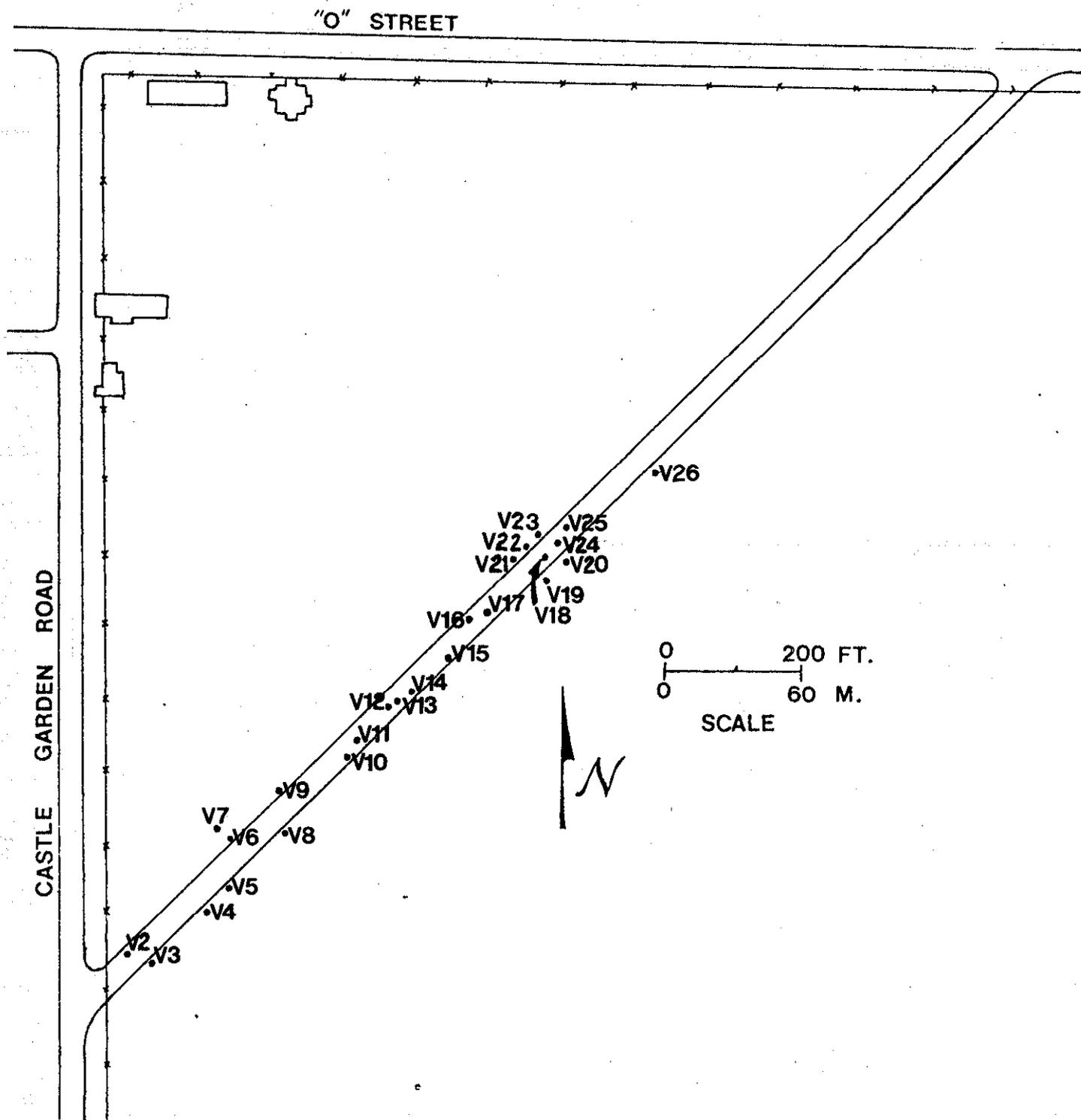
FIGURE 14. Locations of Elevated Surface Contact Radiation Levels Along Vine Street Measured After Remedial Action But Prior to Removal of Additional Soil.
