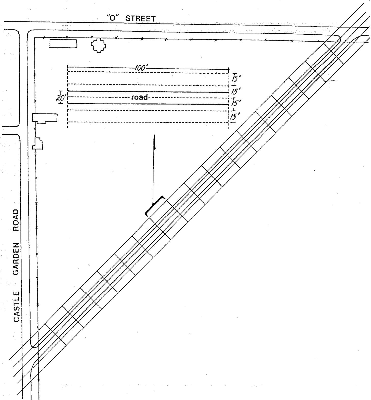
FIGURE 5. Area of Vine Street Showing Grid System Established For Post Remedial Action Survey.
