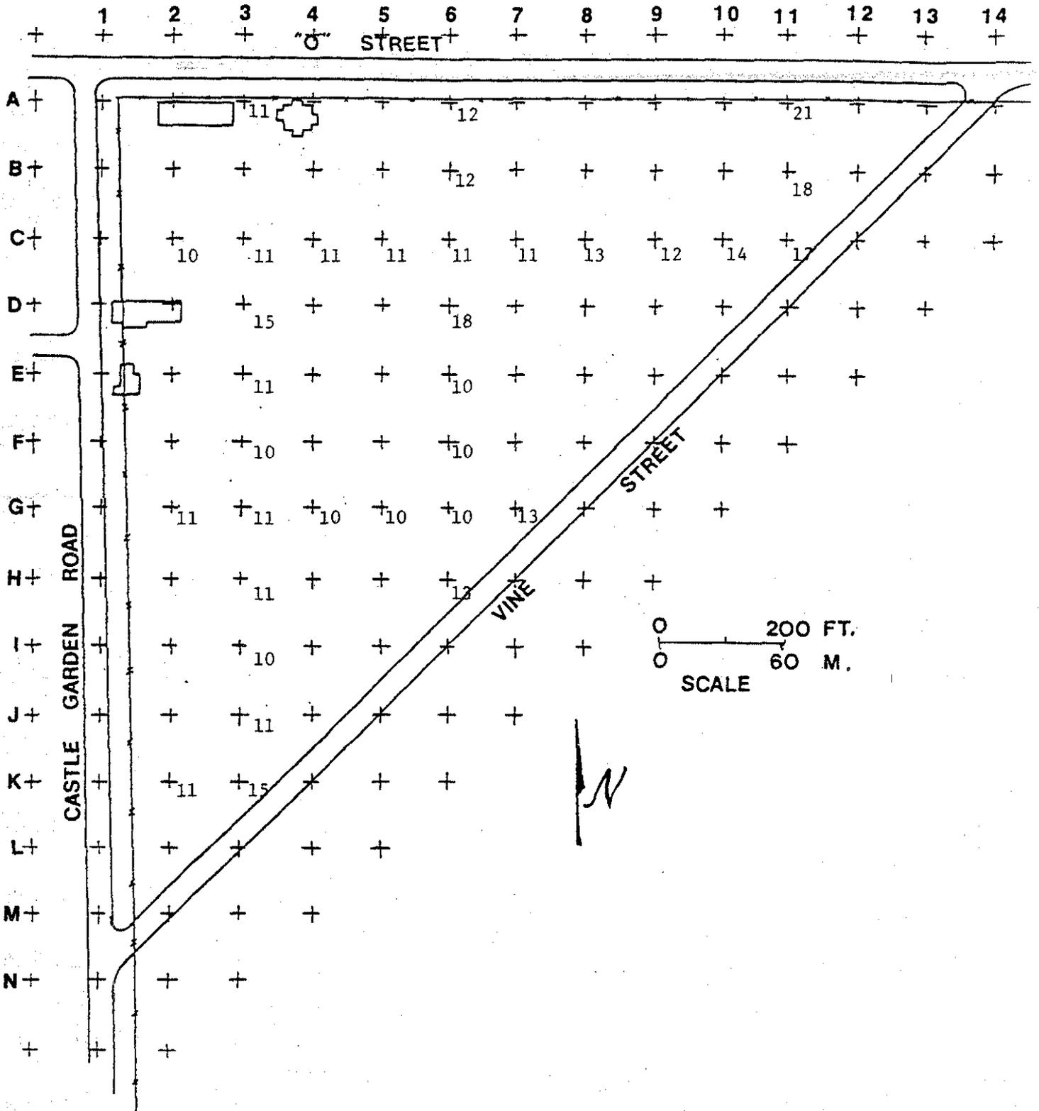
FIGURE 9. Exposure Rates ( $\mu\text{R/h}$ ) at 1 Meter Above the Surface Along Grid Lines C, G, K, 3, 6, and 11: Measurements to Confirm Results of the January 1981 Survey.
