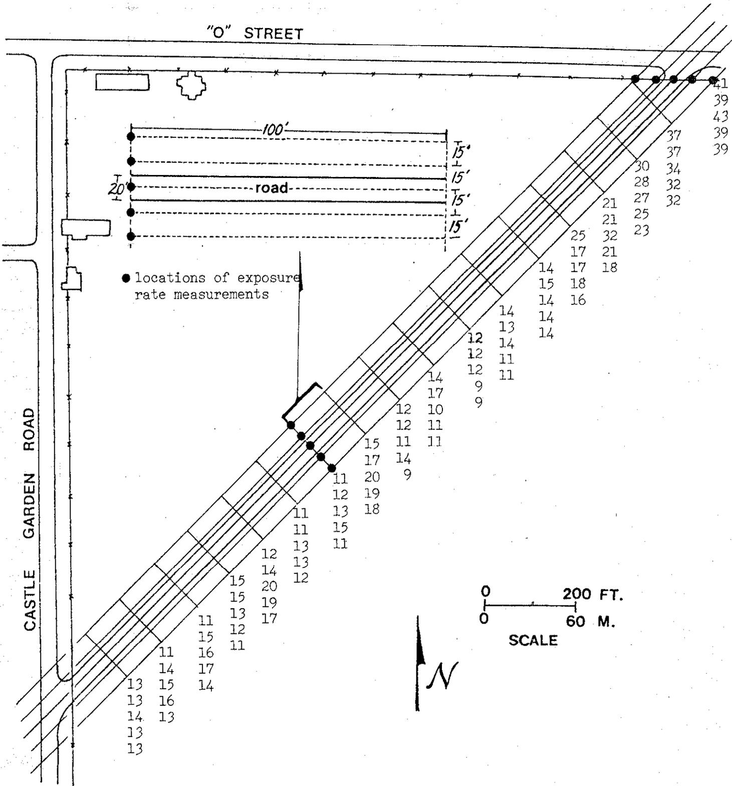
FIGURE 15. Exposure Rates ( $\mu\text{R}/\text{h}$ ) at 1 Meter Above the Surface, Measured Along Vine Street.
