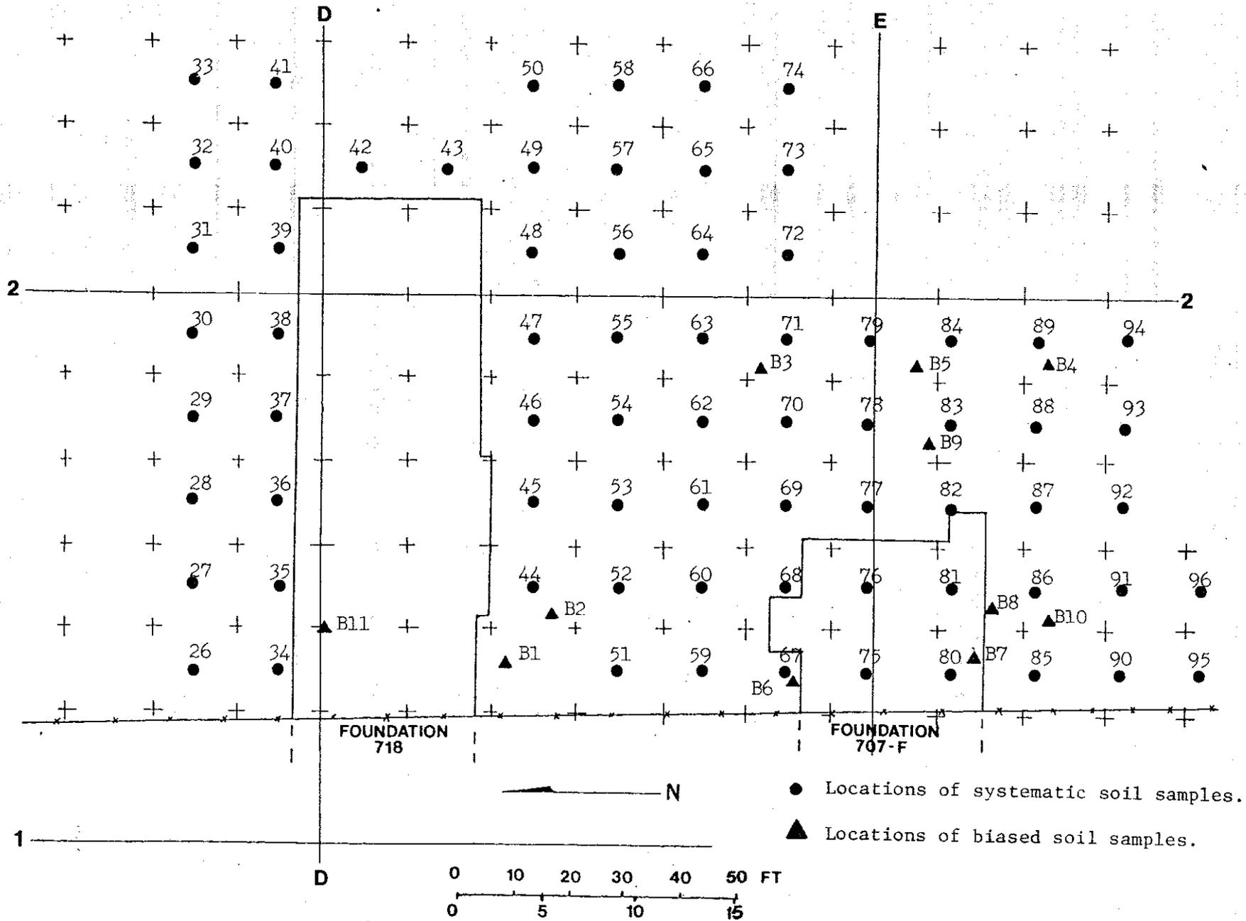
FIGURE 7. Area of Building Foundations, Indicating Locations of Soil Samples
