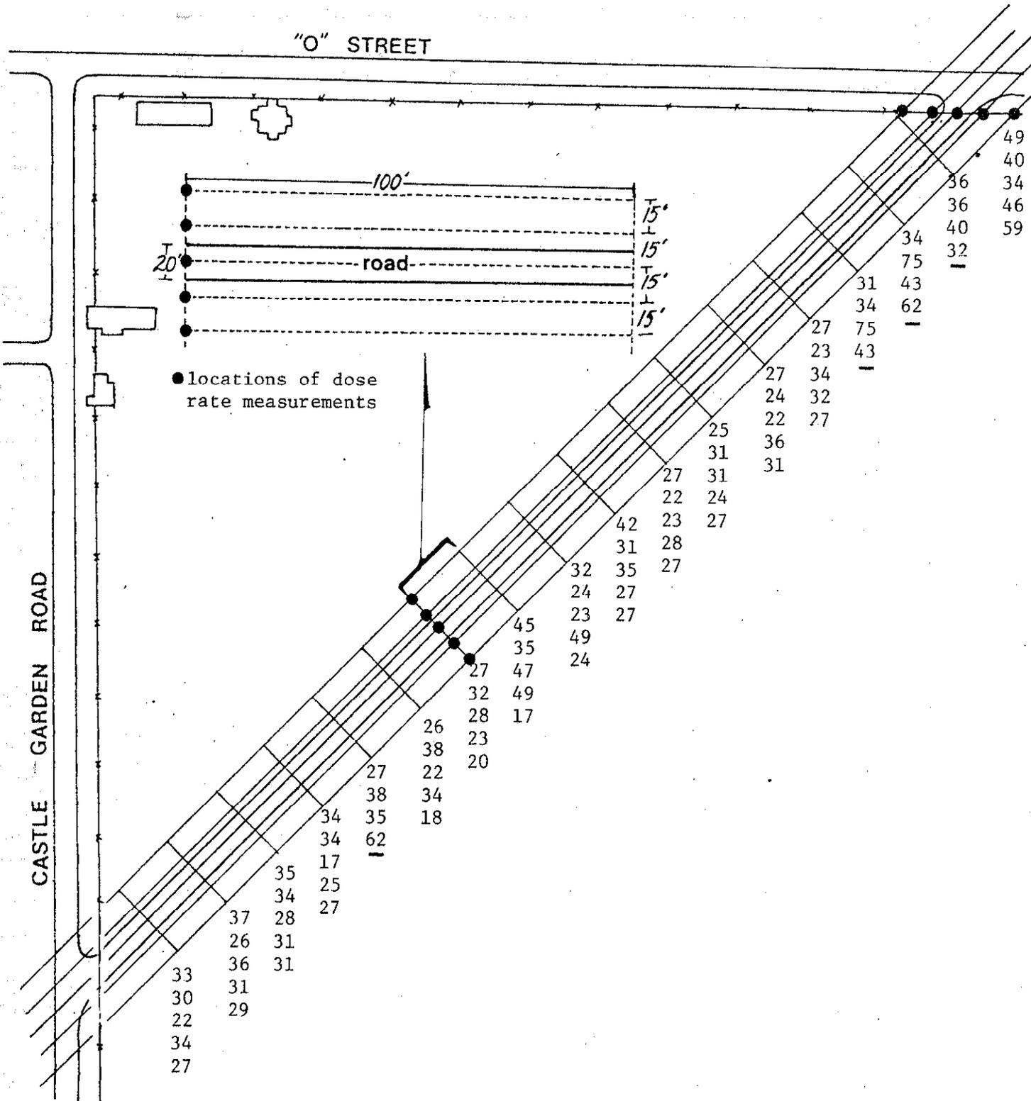
FIGURE 16. Surface Beta-Gamma Dose Rates ( $\mu\text{rad/h}$ ) Measured Along Vine Street.
