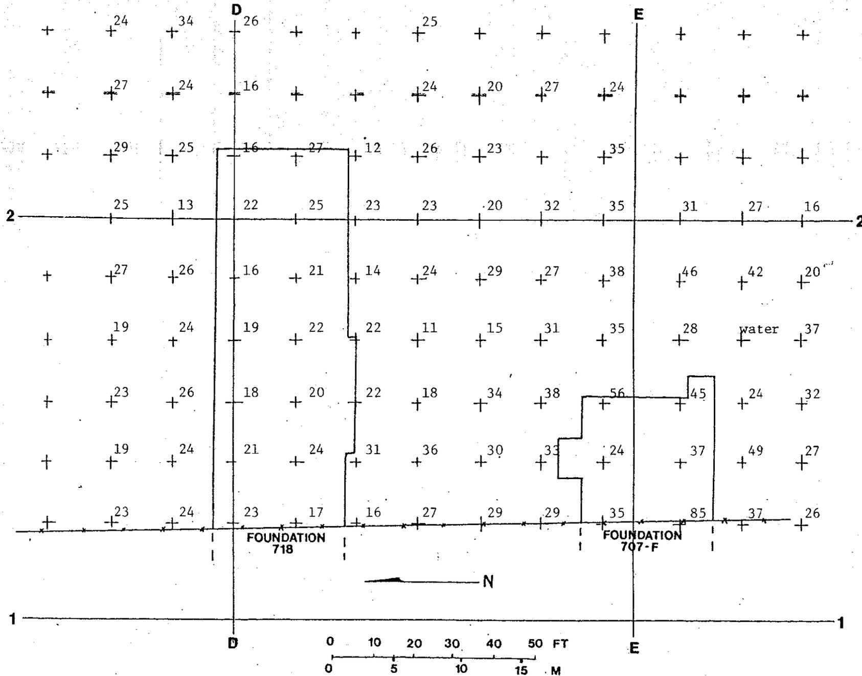
FIGURE 13. Surface Dose Rates ( $\mu\text{rad/h}$ ), Measured in the Vicinity of Building Foundations 718 and 707-F.
