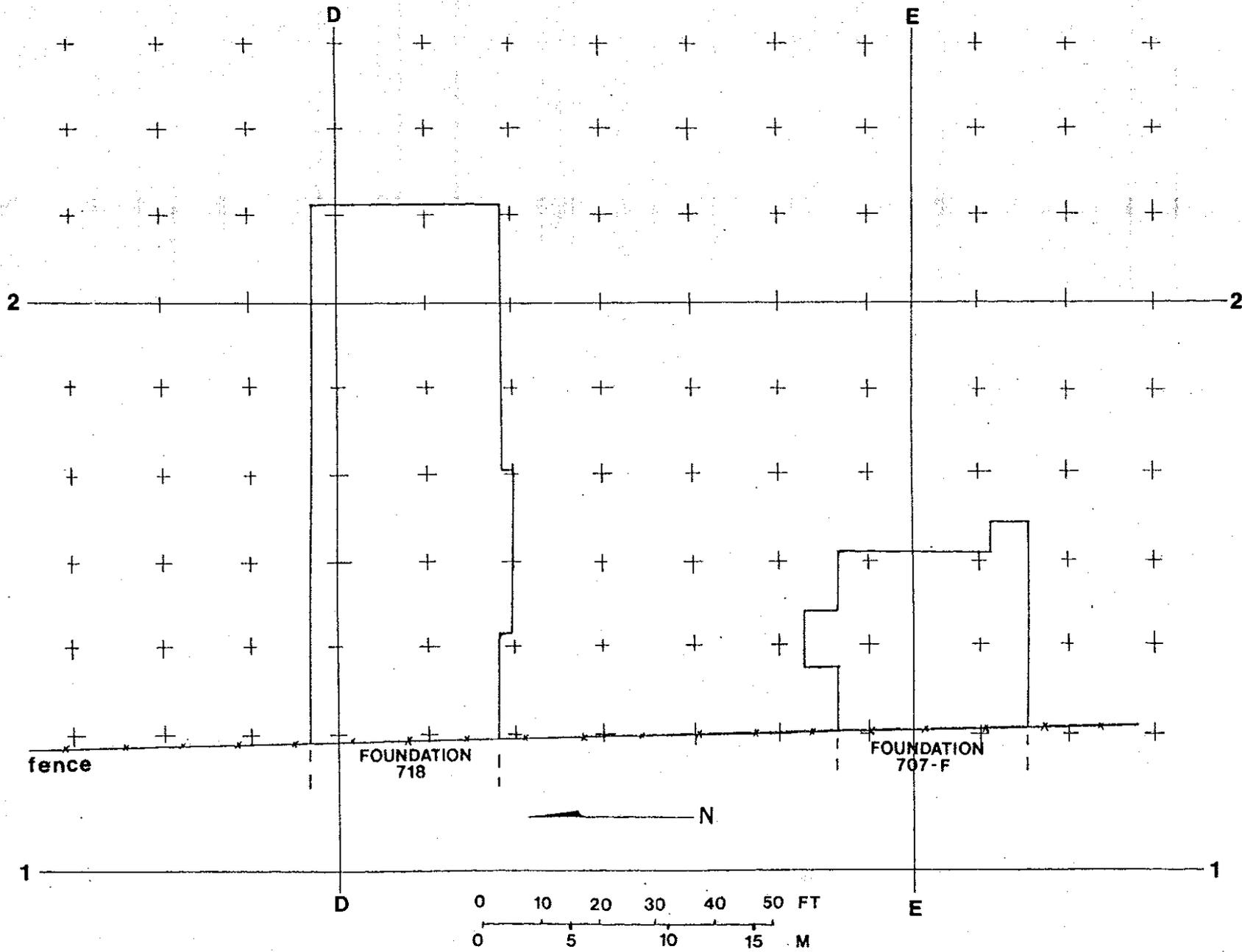
FIGURE 4. Area of Building Foundations 718 and 707-F, Showing 15 foot Grid System for Remedial Action Survey.
