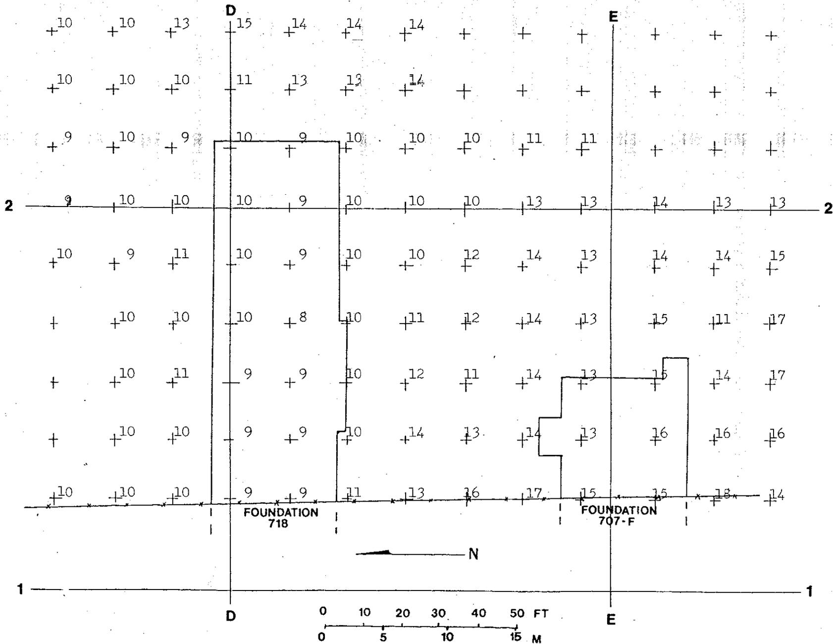
FIGURE 12. Exposure Rates ( $\mu\text{R/h}$ ) at 1 Meter Above the Surface, Measured in the Area of Remedial Action Near the Building Foundations 718 and 707-F.
