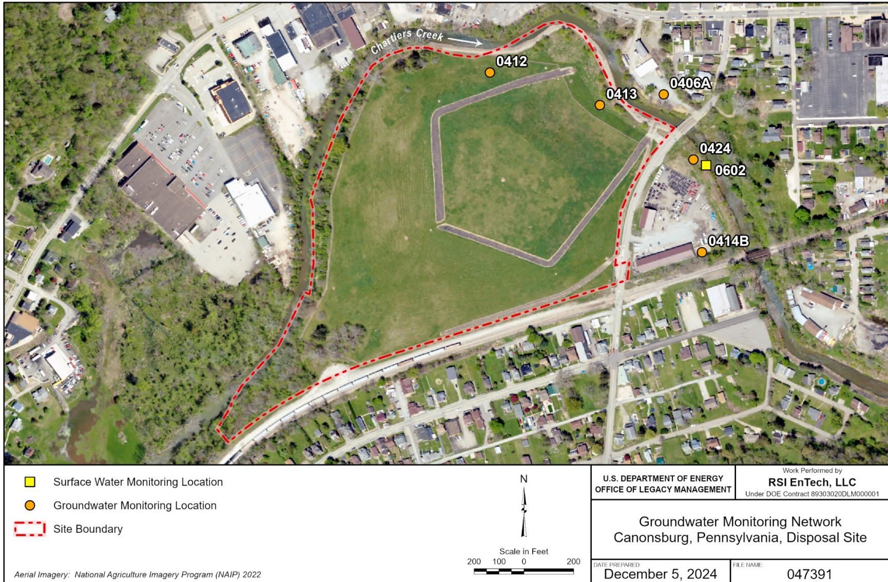
Figure 3-2. Groundwater and Surface Water Monitoring Network for the Canonsburg, Pennsylvania, Disposal Site
