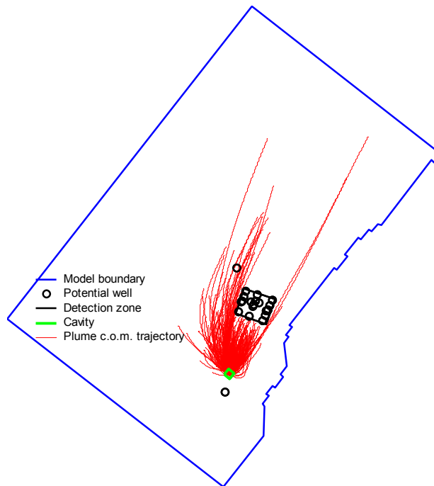
Figure 28. Trajectories of detected plumes superimposed on the potential well locations for the second configuration, where well HC-1 is excluded. Rectangular detection zone and the test cavity are also shown.
