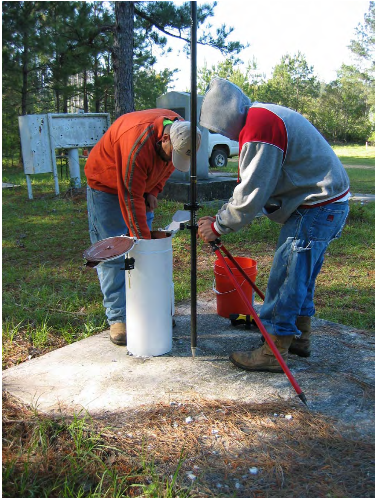
Photo A-6. Surveyors Preparing to Measure Well Elevation
