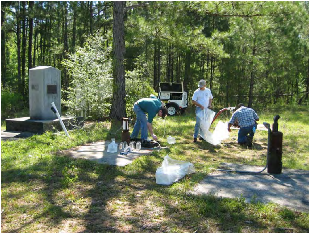
Photo A-5. Monitor Well Sampling by EPA Sampling Team
