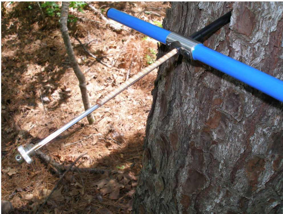
Image A–14. The core sample withdrawn from the incremental borer. The tree rings are visible.
