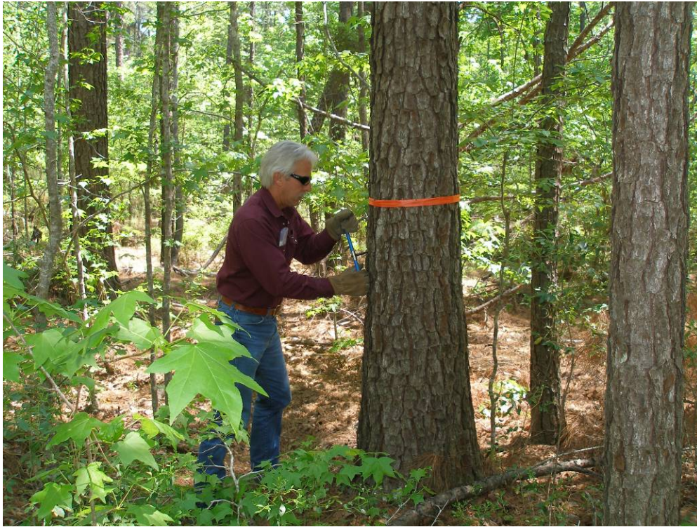
Image A–13. Collection of a tree core sample. The orange tape indicates the tree had previously been sampled by the State.
