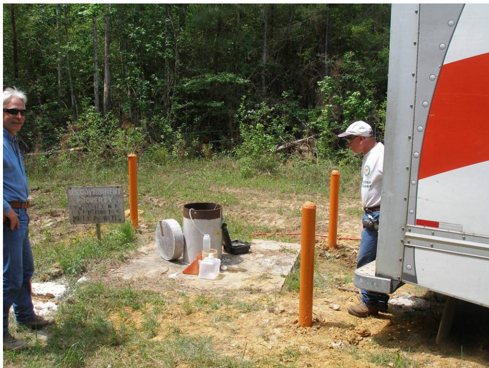
Image A-15. Collection of a groundwater sample at well E-7 by LM.
