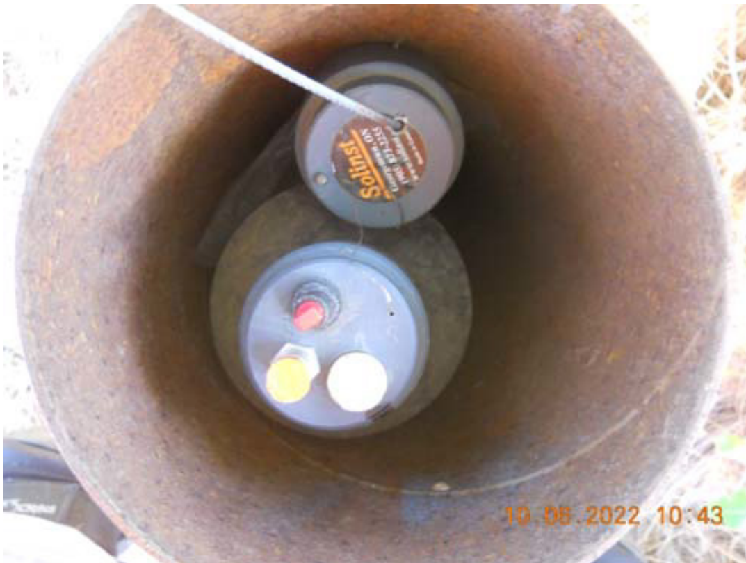
Well UCD1-013: New Water Level Port Plug Installed (Photo No. 4844)
