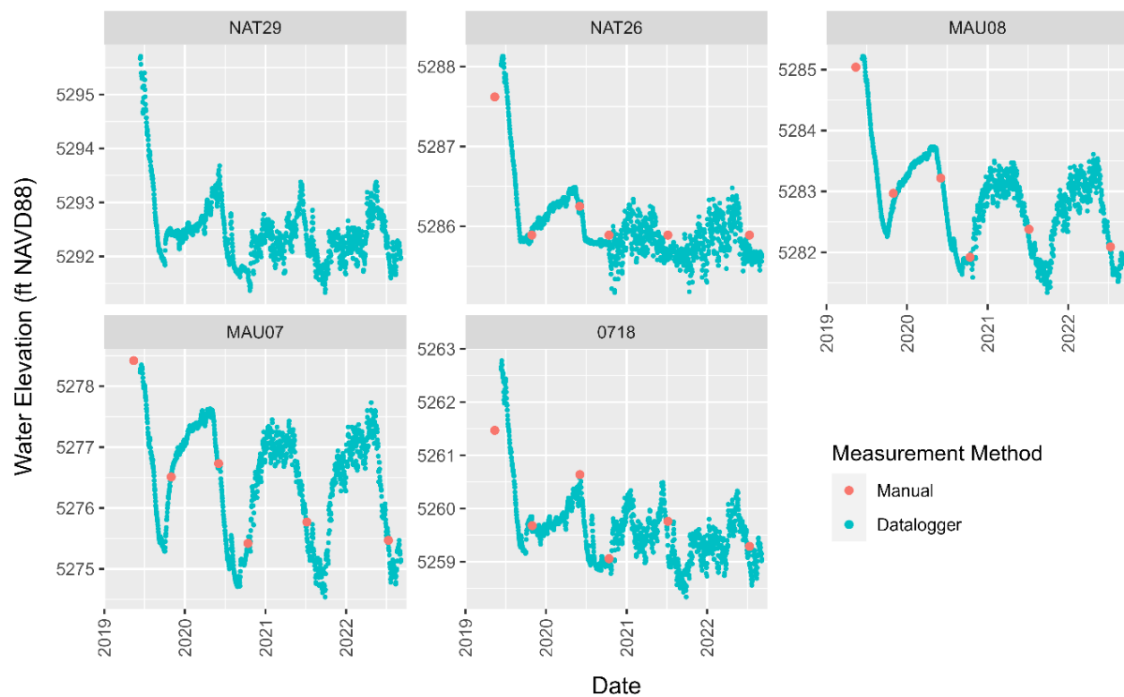
Figure 7. Datalogger Measurements in Selected Wells, June 2019–2022
