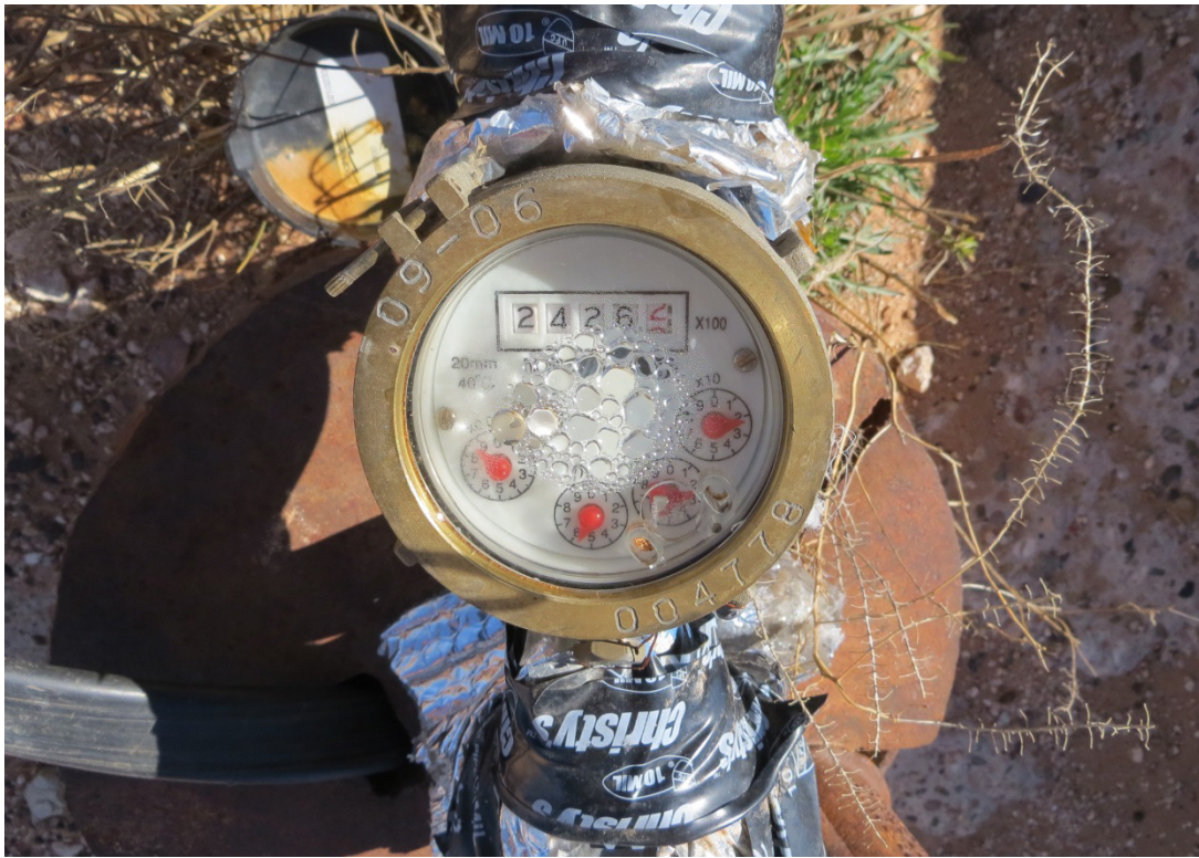
Photograph 1. Flow meter at well USGS-1 showing gallons removed.
