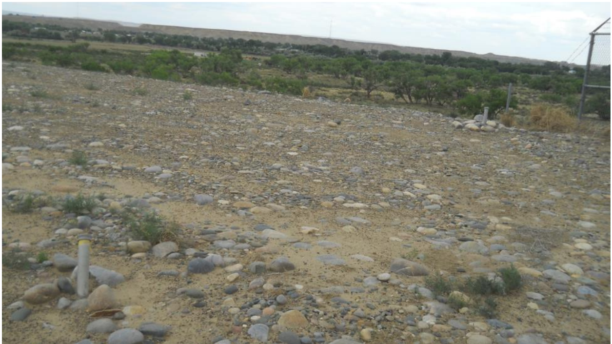
SHP 5/2014. PL-12. Erosion control markers 5A and 5; 5A (foreground) is bent.
