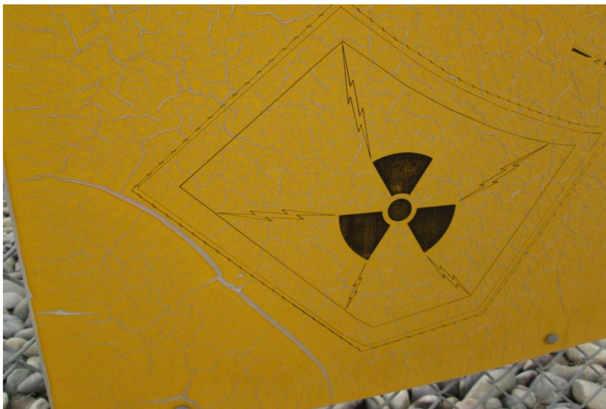
SHP 5/2014. PL-9. Pictorial perimeter sign P4, showing faded and cracked surface.
