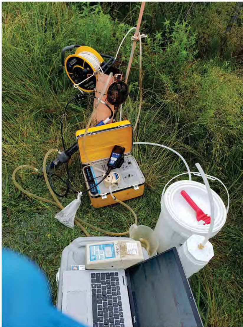
Figure 1. Purging Monitoring Well MW-08S
