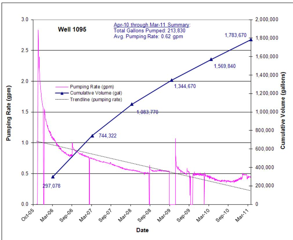
Figure 45. Terrace Well 1095 Pumping Rate and Cumulative Groundwater Volume Extracted
