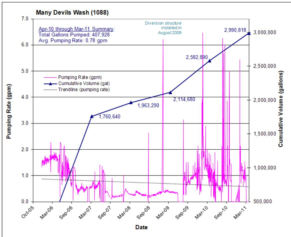
Figure 48. Many Devils Wash Pumping Rate and Cumulative Groundwater Volume Extracted
