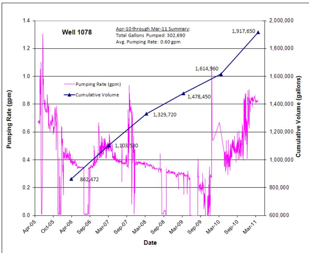
Figure 41. Terrace Well 1078 Pumping Rate and Cumulative Groundwater Volume Extracted
