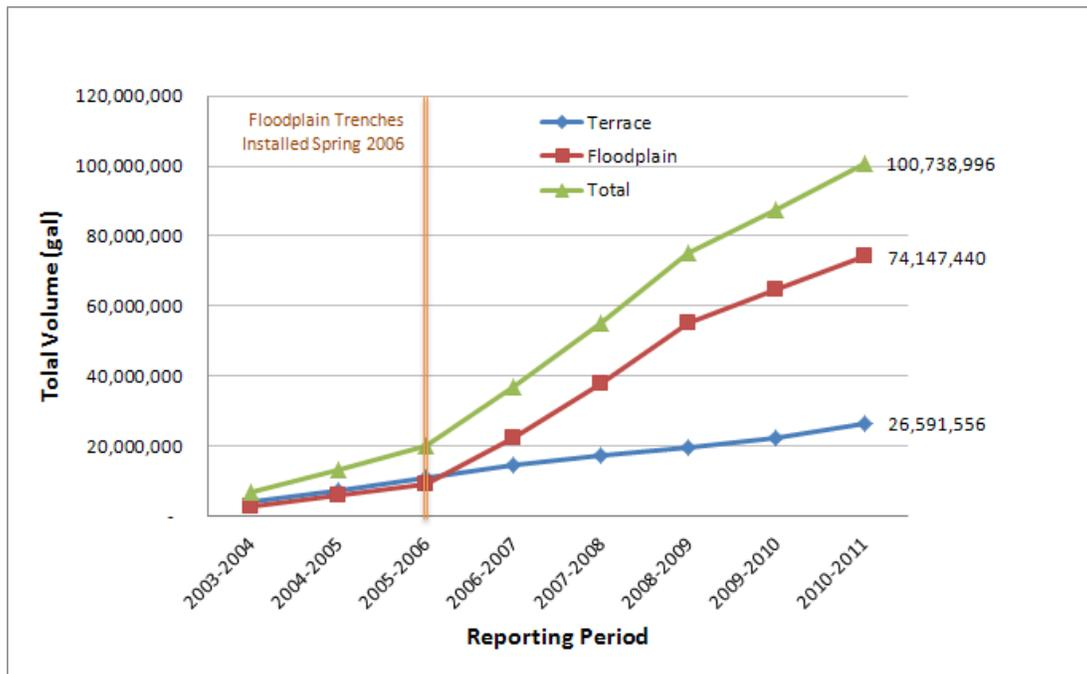
Figure 49. Total Groundwater Volume Pumped to the Evaporation Pond
