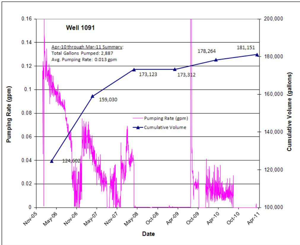
Figure 42. Terrace Well 1091 Pumping Rate and Cumulative Groundwater Volume Extracted
