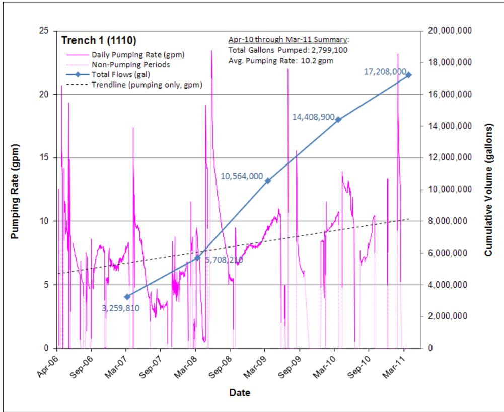
Figure 35. Floodplain Trench 1 Pumping Rate and Cumulative Groundwater Volume Extracted
