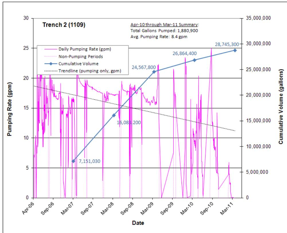
Figure 36. Floodplain Trench 2 Pumping Rate and Cumulative Groundwater Volume Extracted
