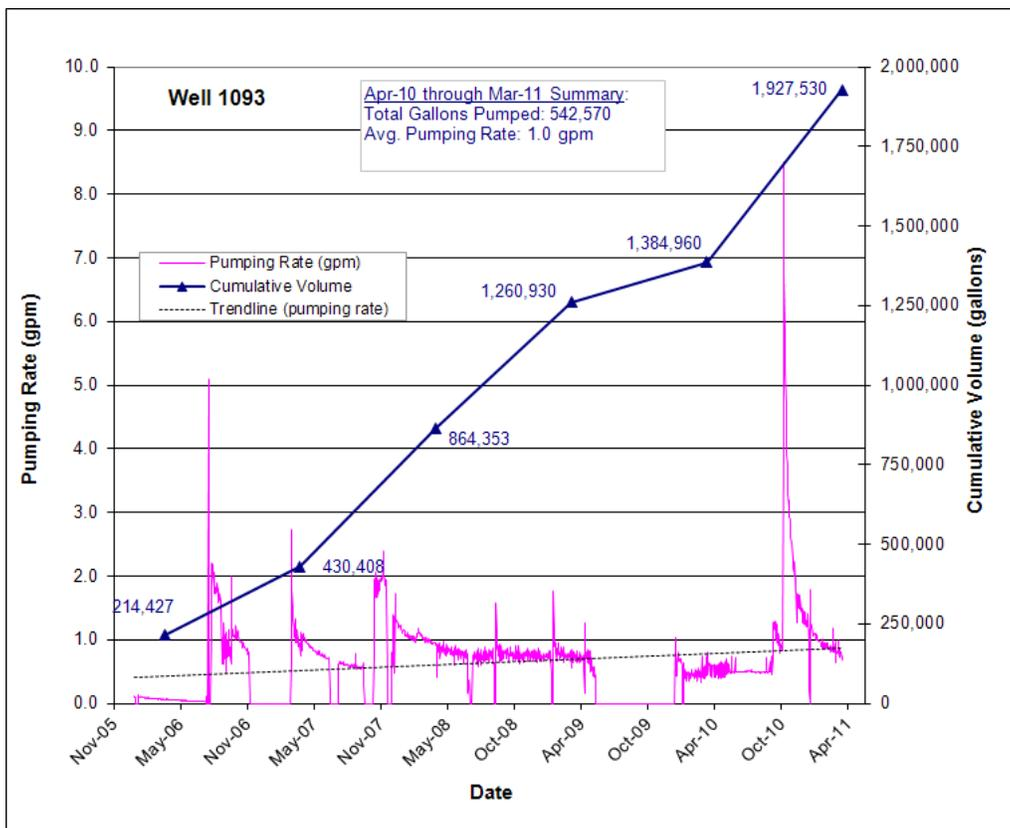
Figure 44. Terrace Well 1093 Pumping Rate and Cumulative Groundwater Volume Extracted
