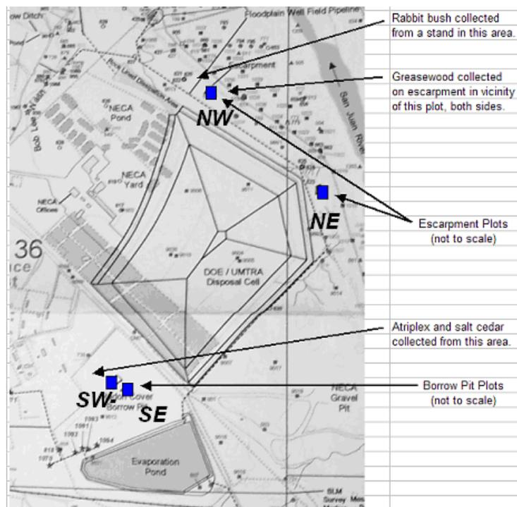
Figure 50. Map of Phytoremediation Test Plots in the Radon Barrier Borrow Pit and on the Terrace above the San Juan River Escarpment
