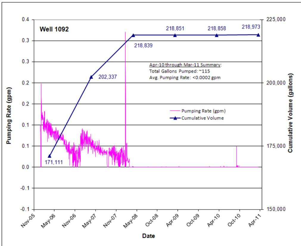
Figure 43. Terrace Well 1092 Pumping Rate and Cumulative Groundwater Volume Extracted
