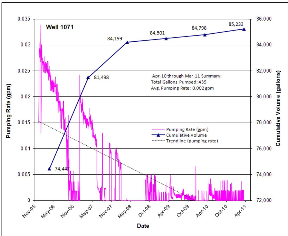
Figure 40. Terrace Well 1071 Pumping Rate and Cumulative Groundwater Volume Extracted
