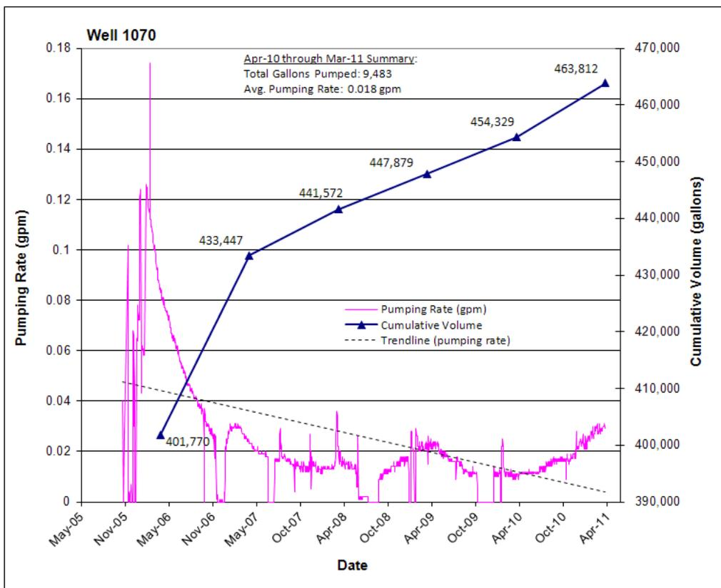
Figure 39. Terrace Well 1070 Pumping Rate and Cumulative Groundwater Volume Extracted
