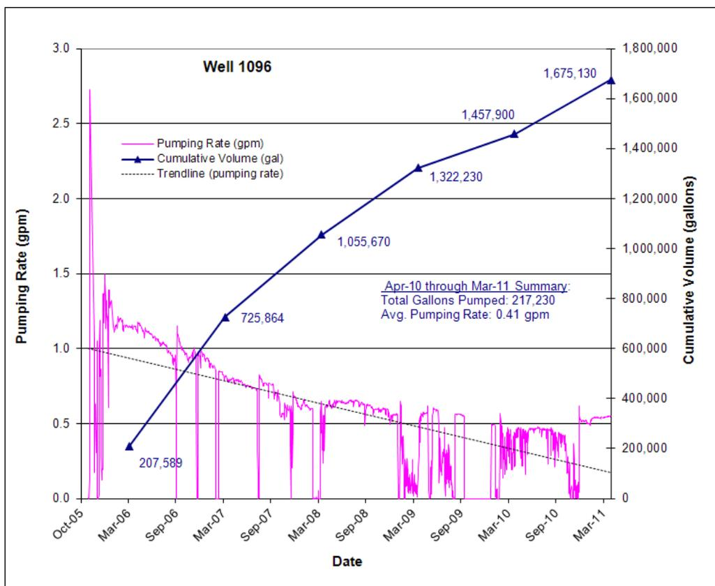
Figure 46. Terrace Well 1096 Pumping Rate and Cumulative Groundwater Volume Extracted
