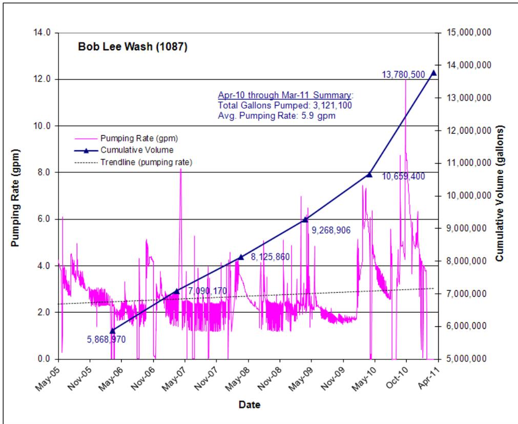
Figure 47. Bob Lee Wash Pumping Rate and Cumulative Groundwater Volume Extracted
