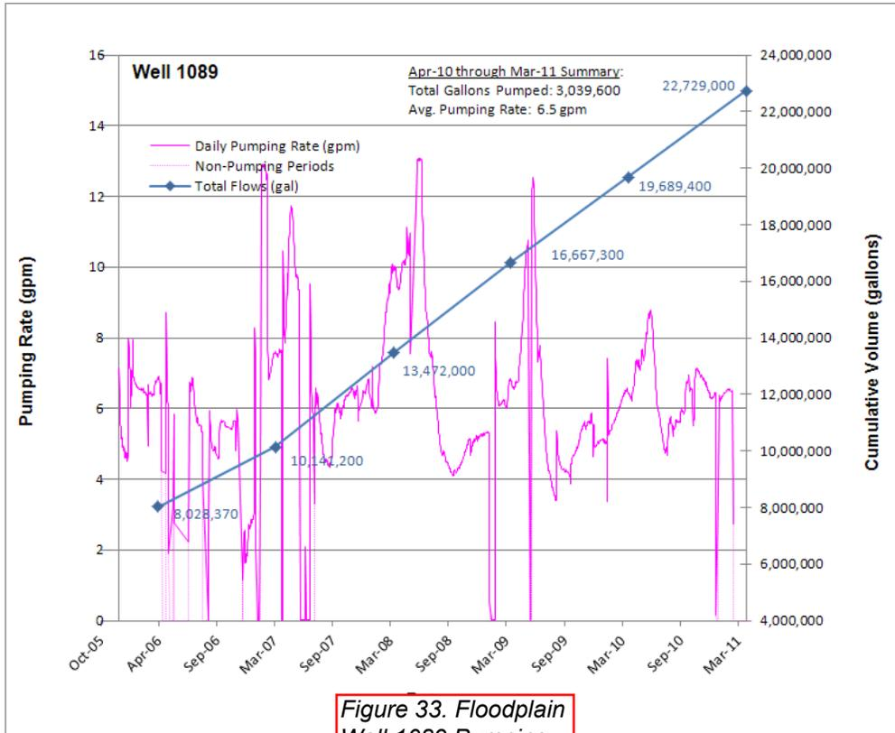
Figure 33. Floodplain Well 1089 Pumping Rate and Cumulative Groundwater Volume Extracted
