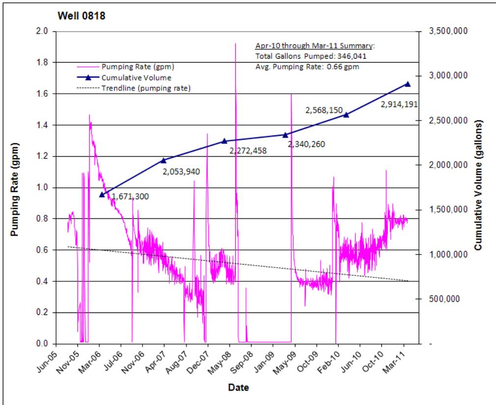
Figure 38. Terrace Well 0818 Pumping Rate and Cumulative Groundwater Volume Extracted
