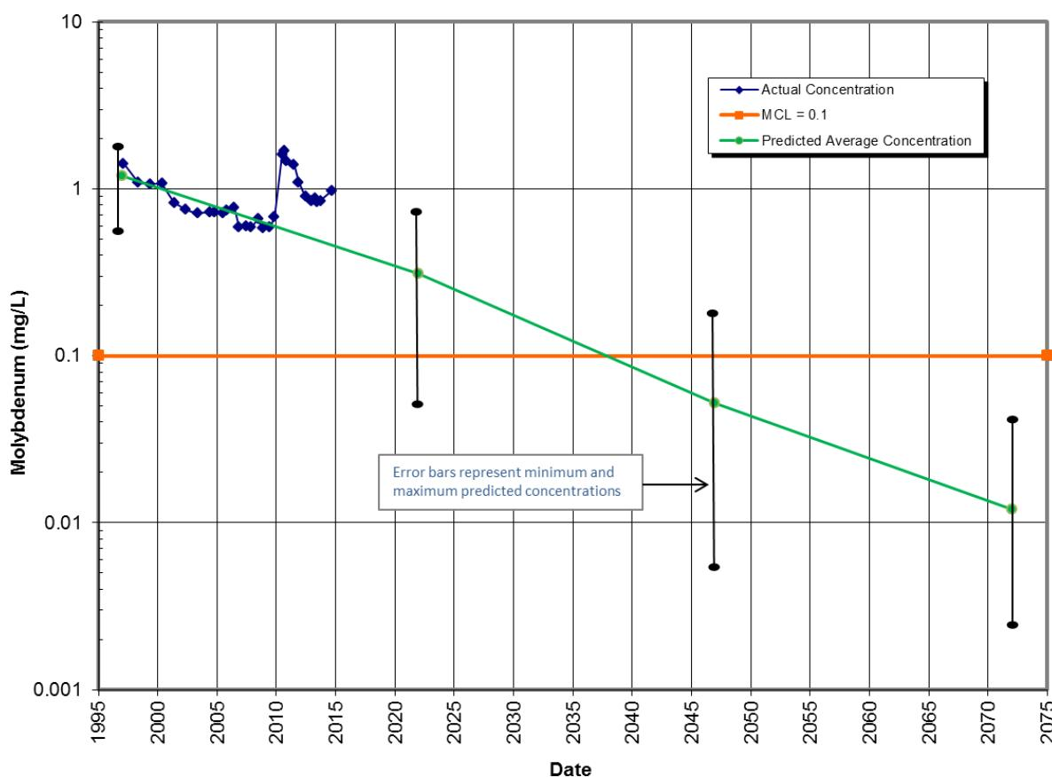
Figure 30. Predicted Versus Actual Molybdenum Concentrations in Well 0707
