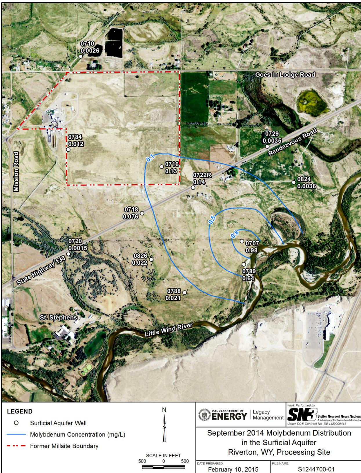
Figure 8. September 2014 Molybdenum Distribution in the Surficial Aquifer at the Riverton Site
