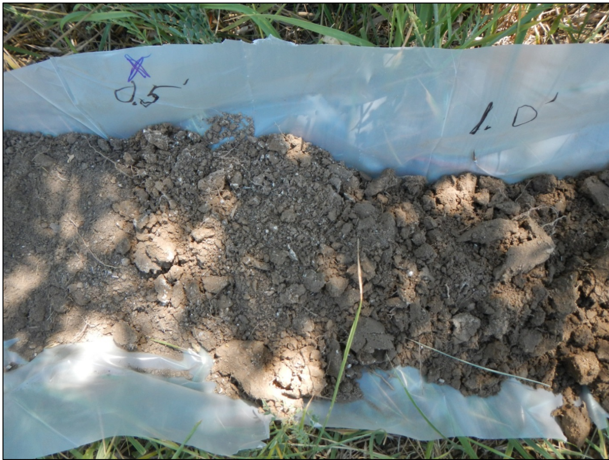
Figure 29. Soil Sample from Location 0882 (depth indicated in feet). White flecks are evaporite.
