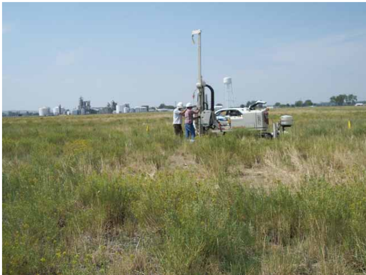
Figure 27. Installing a Borehole with a Geoprobe in August 2012
