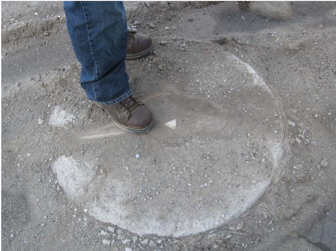
HAL 4/2010. PL-8. Flush mount monitoring well OBS-1B.
