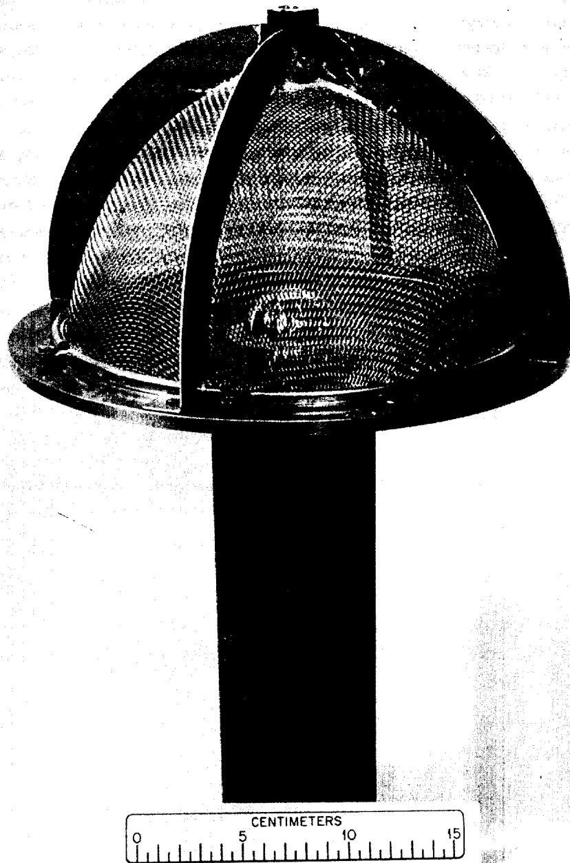
Fig. I-C. View of mylar covered ZnS detector inside ground screen.
