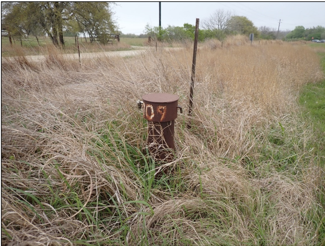
PL-4. Monitoring Well 0709
