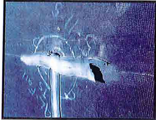
Typical Peel Failure of Extrusion Weld
