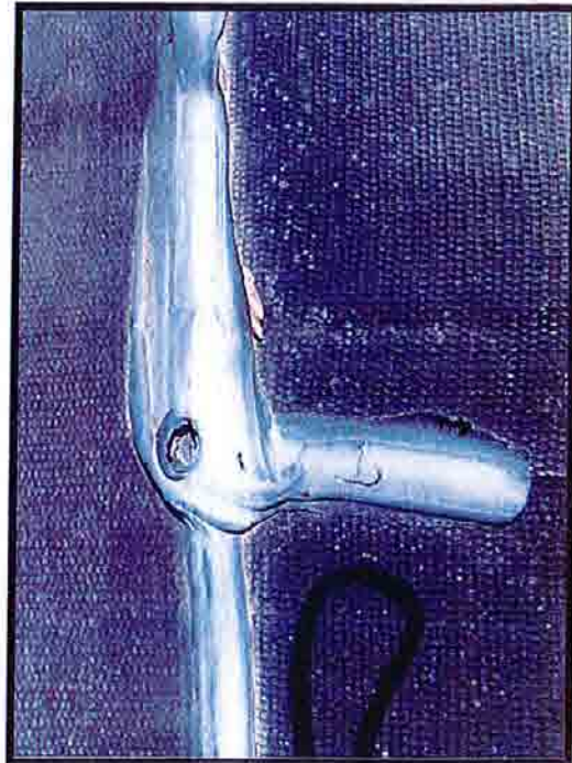
Typical "Bubbling" Failure of Extrusion Weld
