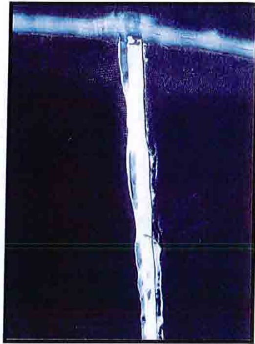
Typical Peel Failure of Extrusion Weld
