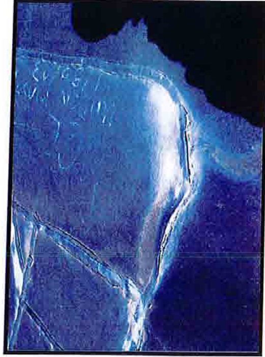
Typical Peel Failure of Extrusion Weld
