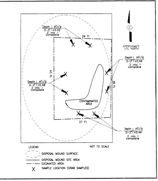
by 5 m by 0.3 m (19.5 ft by 16 ft by 1 ft). The contaminated soil was removed manually with shovels and placed in four B-25 containers. Approximately 9 m<sup>3</sup> (12 yd<sup>3</sup>) of soil were removed; this amount is based on the dimensions of the excavated area and the approximate depth to which the soil was removed. The area was then resurveyed with the Eberline ESP-2/Nal ratemeter. This survey indicated only background levels of naturally occurring radioisotopes.
