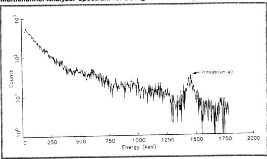
Figure 5-11 Multichannel Analyzer Spectrum for Background Area D (near Mound)
