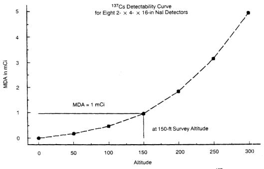
FIGURE B-2. MINIMUM DETECTABLE ACTIVITY CURVE FOR 137Cs
