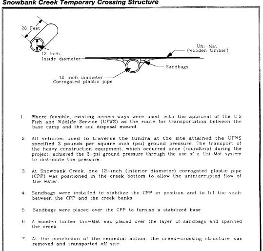
Figure 6-2 Snowbank Creek Temporary Crossing Structure
