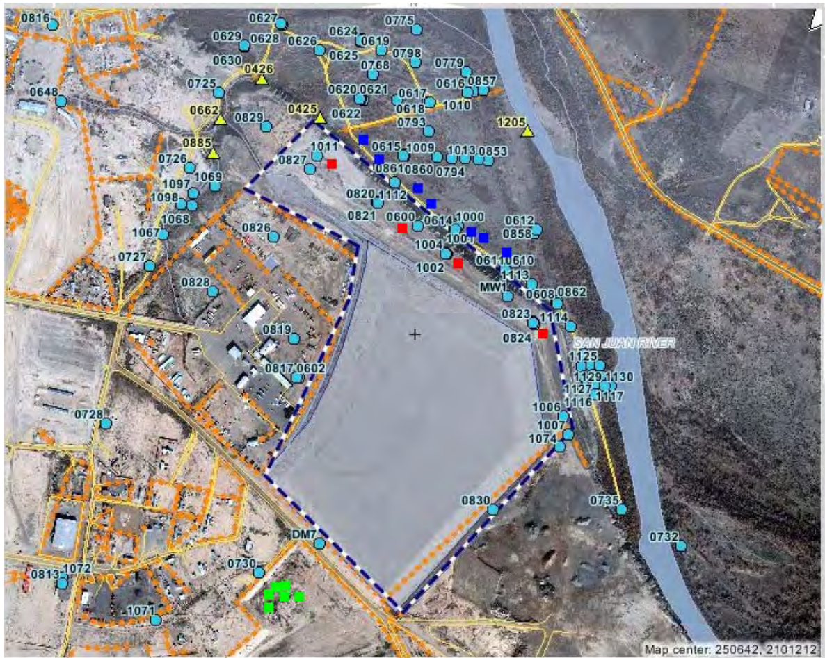
Figure 3–3. Map of wells and approximate location of plant samples. Green squares show where Atriplex canescens (ATCA) and Tamarix ramosissima (TARA) were sampled in the borrow pit area. Red squares show where Sarcobatis vermiculatus (SAVE) was sampled along the cell escarpment. Blue squares show where TARA plants were sampled in the floodplain below the cell.
