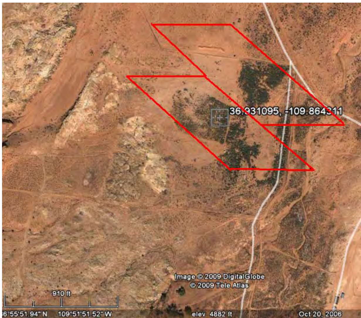
Figure 6–7. MODIS pixel footprints superimposed on a Quickbird image showing the irrigated field and volunteer ATCA stand inside the fence at the Monument Valley site.
