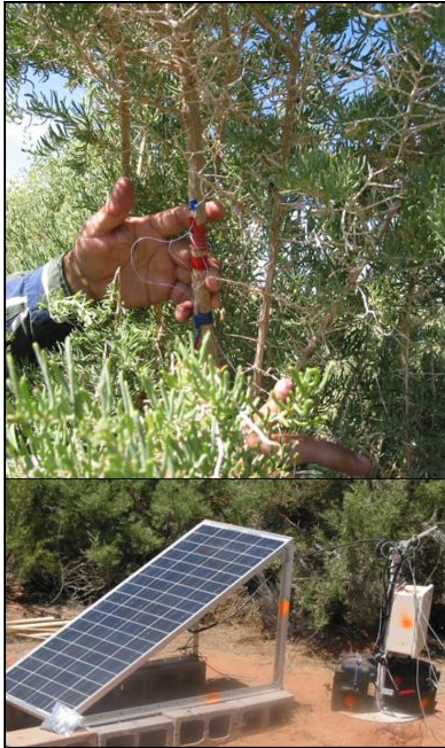
Figure C-8. Wiring for a heat-dissipation stem flow sensor on a black greasewood ( Sarcobatus vermiculatus ) plant rooted in the alluvial aquifer at the Monument Valley site (top photo), and photovoltaic panel, batteries, and datalogger to power and record data from the stem flow sensor (bottom photo).
