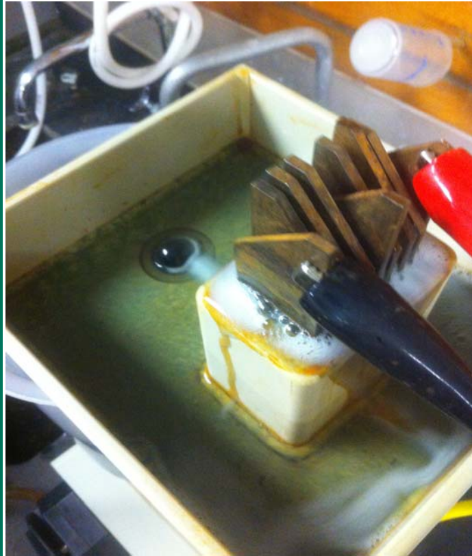
PHOTO 3 Bench EC unit in operation
