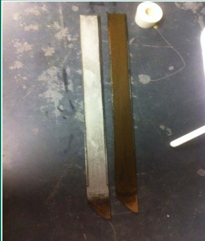
PHOTO 4 Comparison of clean (left) and dirty (right) blades
