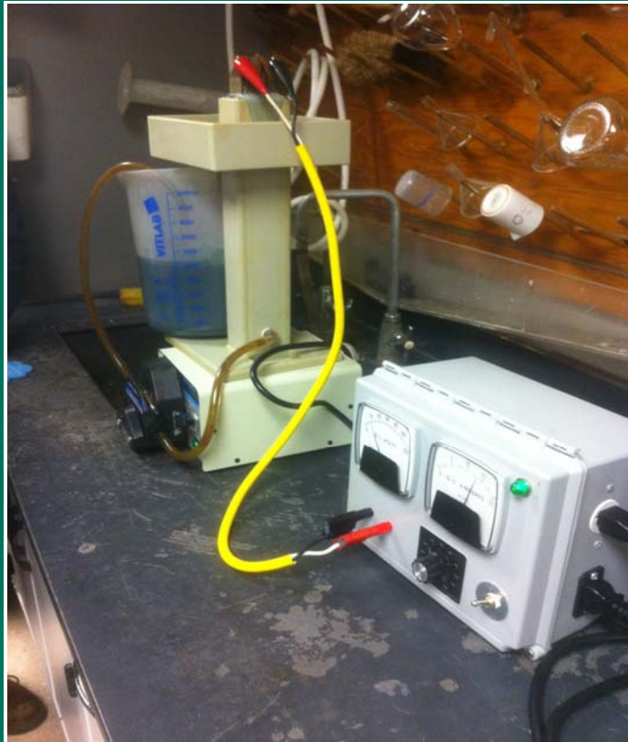
PHOTO 1 Electrocoagulation 1- L Bench-scale Unit with Iron Blades Installed
