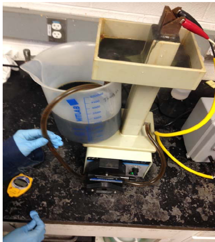
PHOTO 1 Bench EC unit in operation
