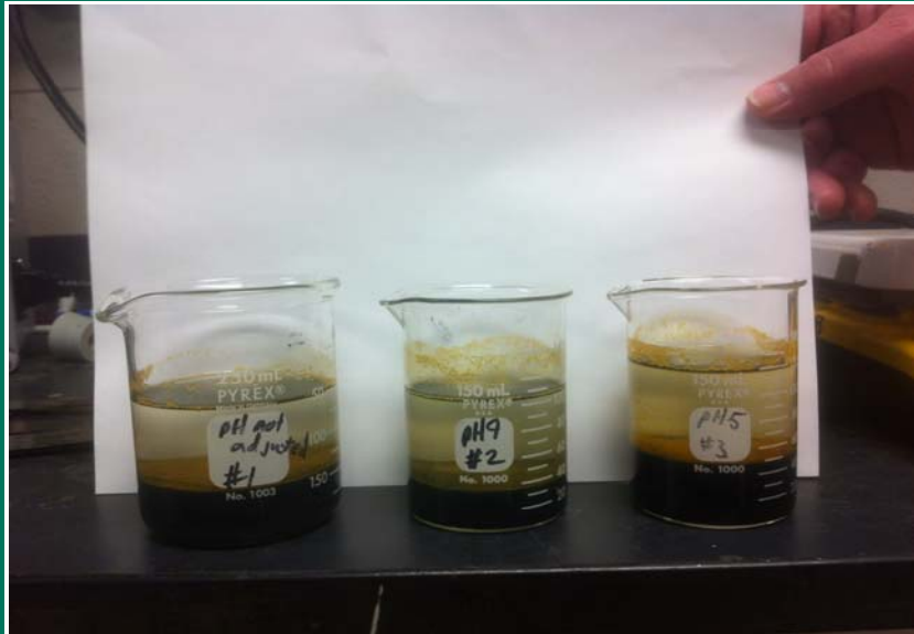
PHOTO 5 High TDS groundwater after 1 minute of treatment with pH adjustment, after settling. As- received pH (left), pH 9 (center), pH 5 (right).
