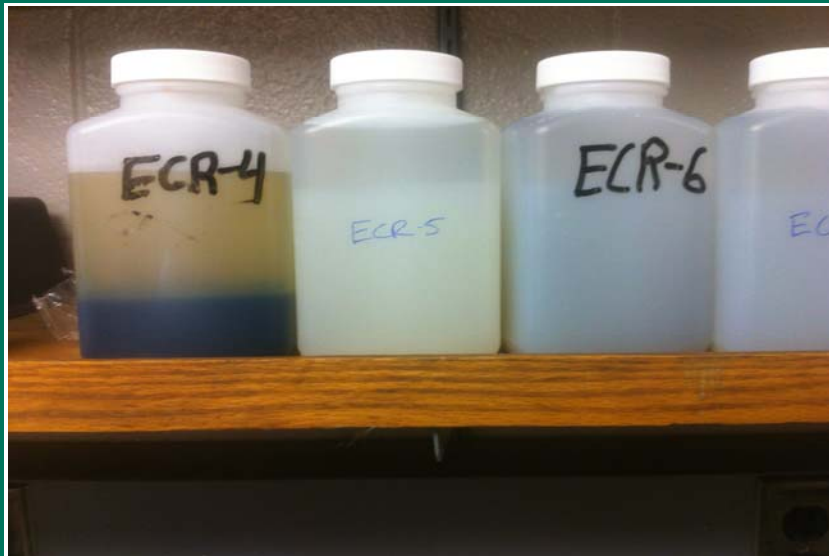
PHOTO 6 Comparison of EC treatment with Iron Blades and Aluminum Blades
