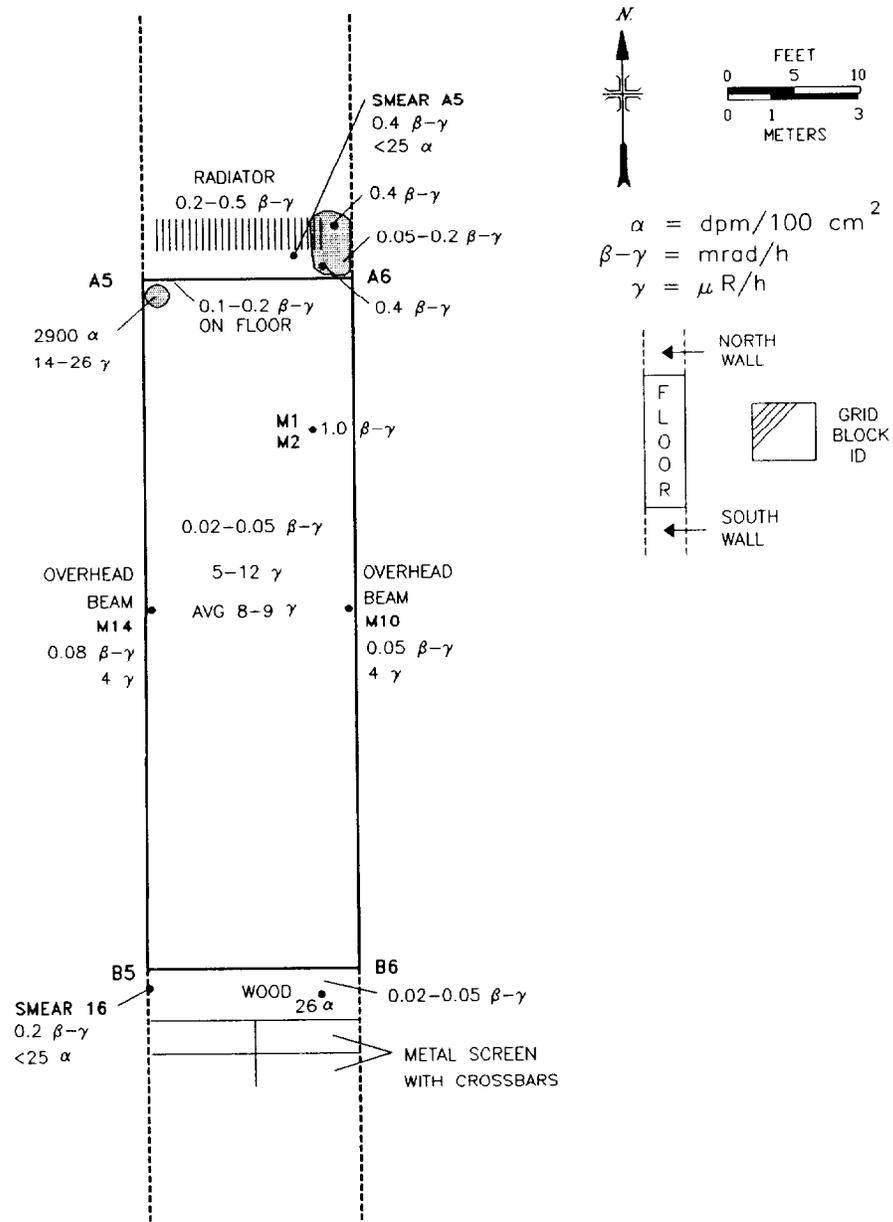
Fig. 13. Surface gamma exposure rates ( $\mu\text{R}/\text{h}$ ), beta-gamma dose rates (mrad/h), and alpha activity levels (dpm/100  $\text{cm}^2$ ) in grid block A5.
