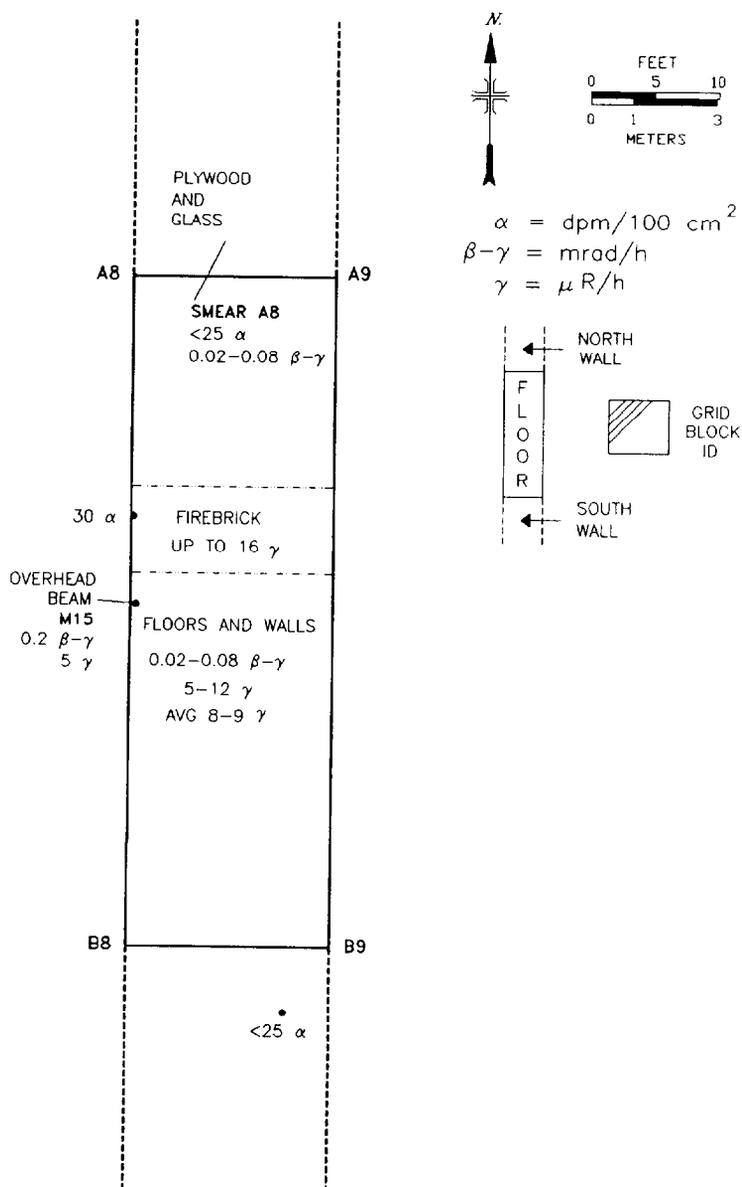
Fig. 16. Surface gamma exposure rates ( $\mu\text{R}/\text{h}$ ), beta-gamma dose rates ( $\text{mrad}/\text{h}$ ), and alpha activity levels ( $\text{dpm}/100 \text{ cm}^2$ ) in grid block A8.
