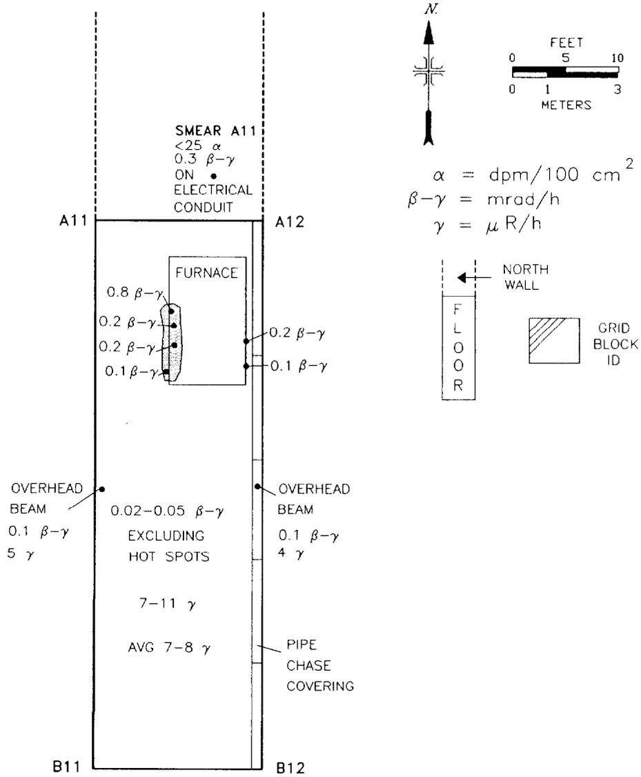
**Fig. 18. Surface gamma exposure rates ( $\mu\text{R/h}$ ), beta-gamma dose rates (mrad/h), and alpha activity levels (dpm/100  $\text{cm}^2$ ) in grid block A11.**
