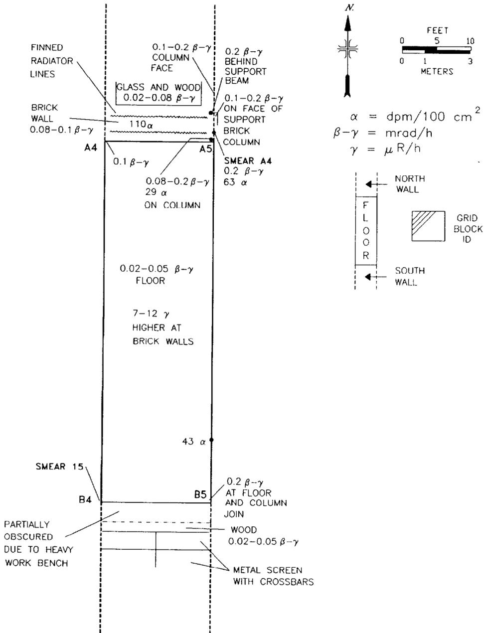
**Fig. 12. Surface gamma exposure rates ( $\mu\text{R}/\text{h}$ ), beta-gamma dose rates ( $\text{mrad}/\text{h}$ ), and alpha activity levels ( $\text{dpm}/100 \text{ cm}^2$ ) in grid block A4.**
