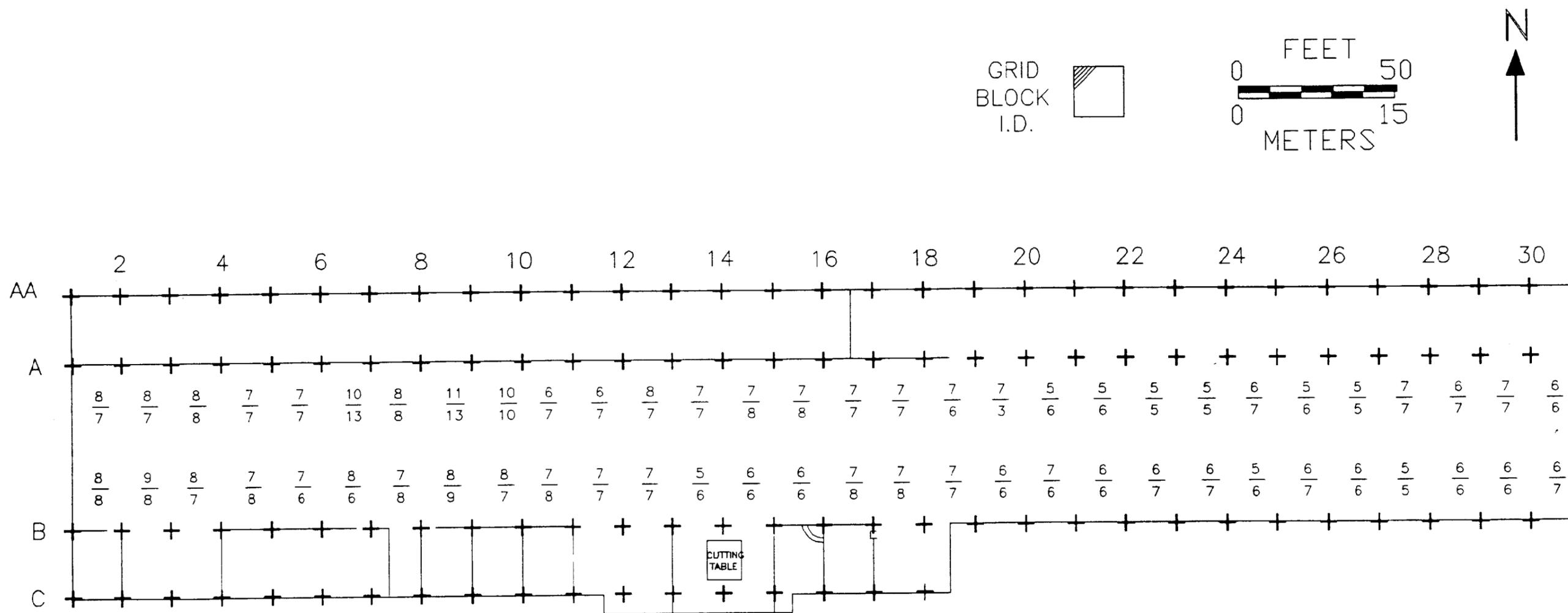
Fig. 5. Surface and 1-m gamma exposure rates ( $\mu R/h$ ) taken at the center of the north and south sections of grid blocks A1 through A30, Building 23, Indian Orchard, Massachusetts. Lower number = surface; upper number = 1 m.
