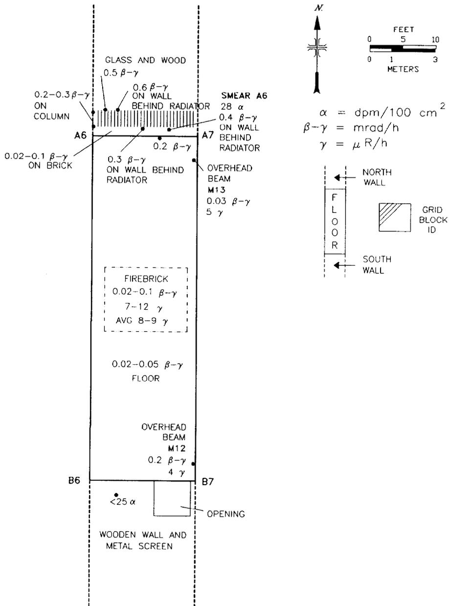
Fig. 14. Surface gamma exposure rates ( $\mu\text{R/h}$ ), beta-gamma dose rates ( $\text{mrad/h}$ ), and alpha activity levels ( $\text{dpm}/100\text{ cm}^2$ ) in grid block A6.
