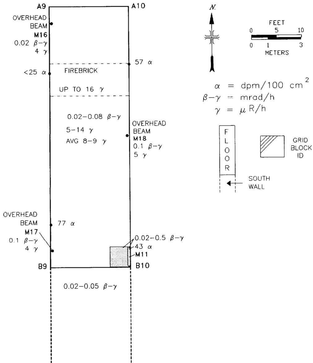
Fig. 17. Surface gamma exposure rates ( $\mu\text{R/h}$ ), beta-gamma dose rates (mrad/h), and alpha activity levels (dpm/100  $\text{cm}^2$ ) in grid block A9.
