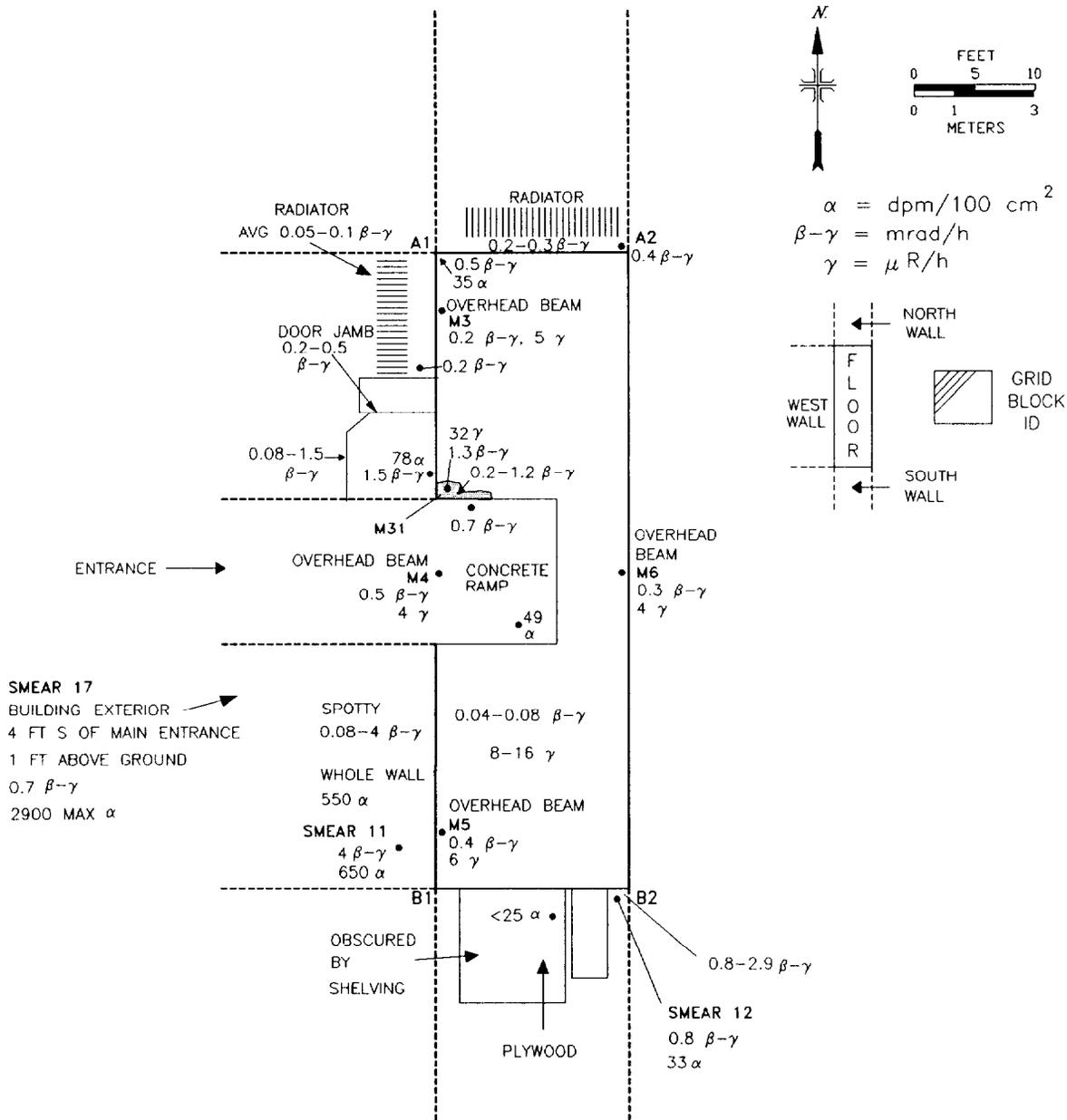
Fig. 9. Surface gamma exposure rates ( $\mu\text{R/h}$ ), beta-gamma dose rates (mrad/h), and alpha activity levels (dpm/100  $\text{cm}^2$ ) in grid block A1.
