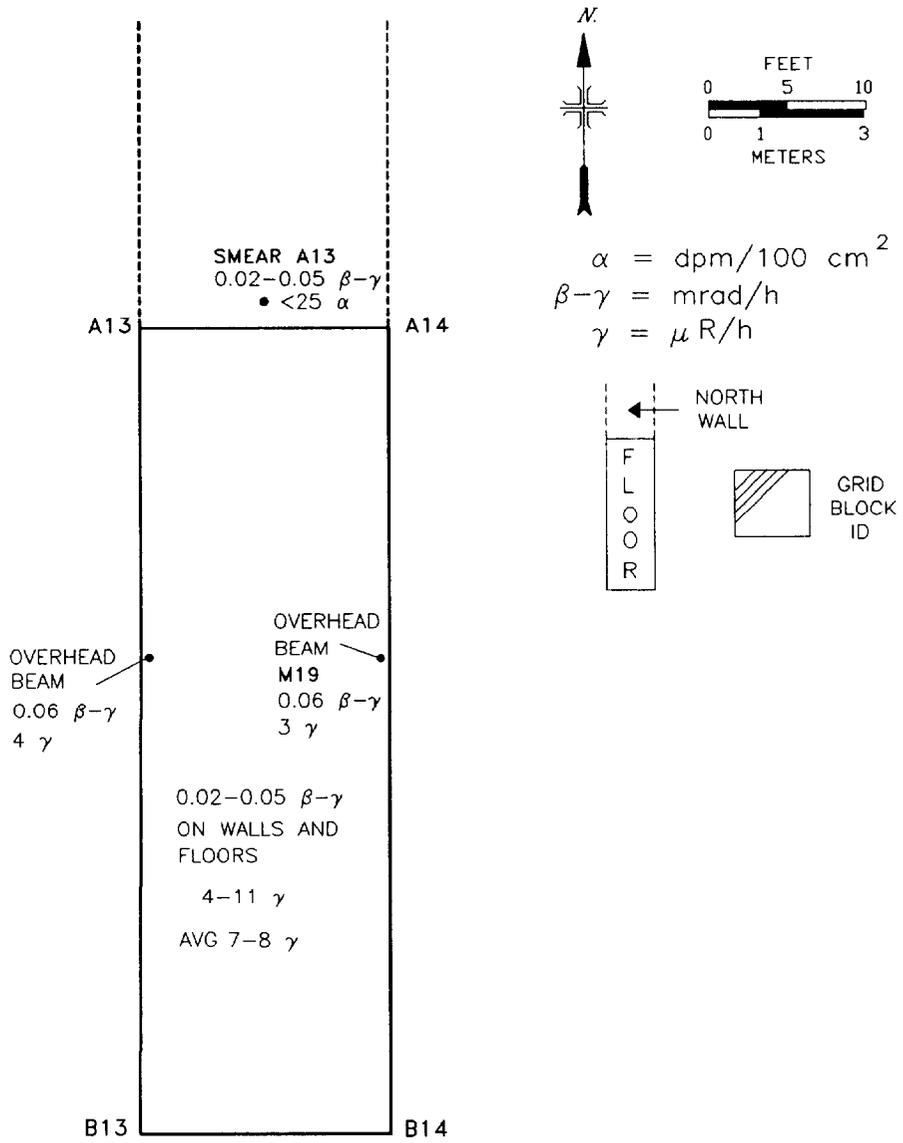
**Fig. 19. Surface gamma exposure rates ( $\mu$ R/h), beta-gamma dose rates (mrad/h), and alpha activity levels (dpm/100 cm<sup>2</sup>) in grid block A13.**
