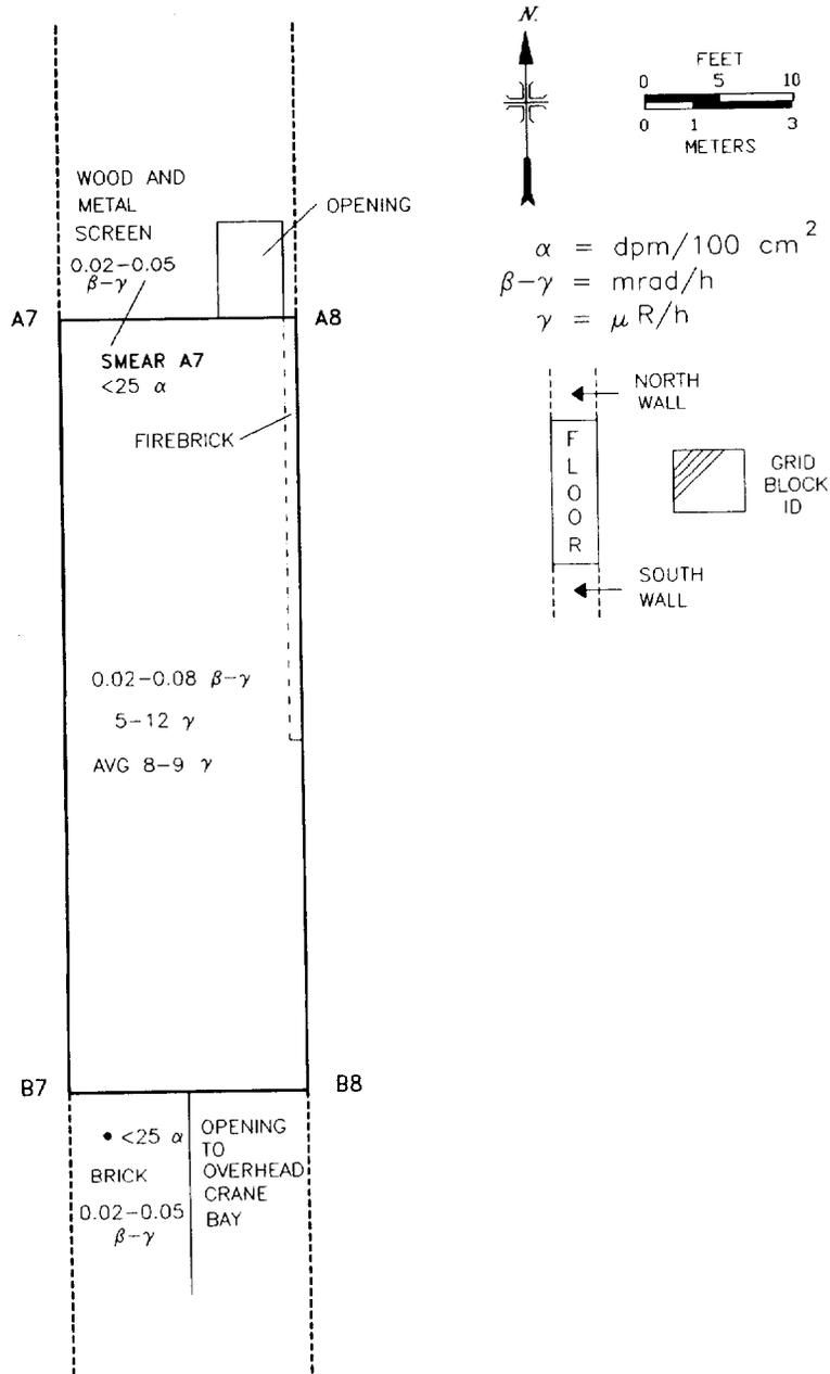
Fig. 15. Surface gamma exposure rates ( $\mu$ R/h), beta-gamma dose rates (mrad/h), and alpha activity levels (dpm/100 cm<sup>2</sup>) in grid block A7.
