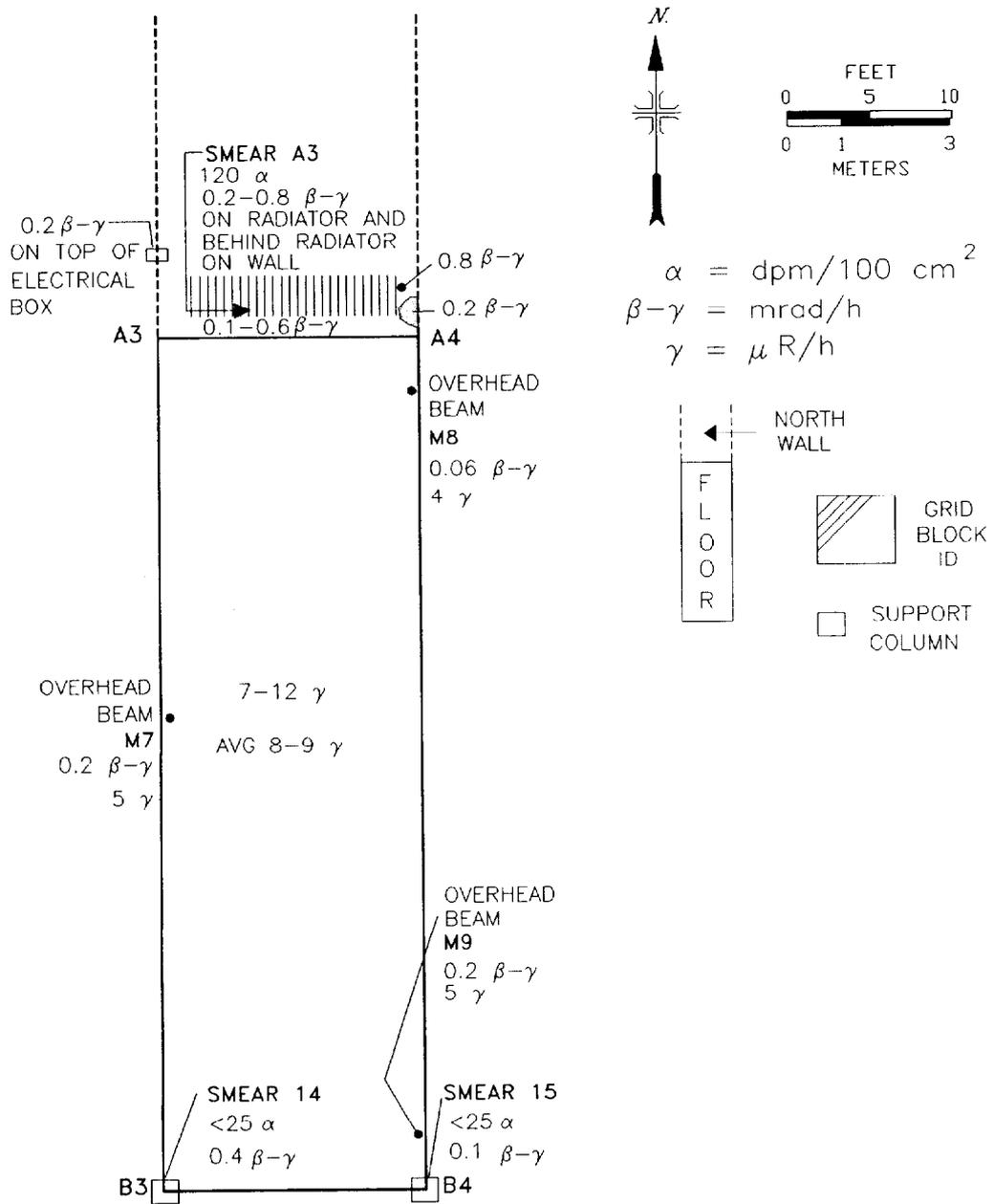
Fig. 11. Surface gamma exposure rates ( $\mu\text{R/h}$ ), beta-gamma dose rates (mrad/h), and alpha activity levels (dpm/100  $\text{cm}^2$ ) in grid block A3.
