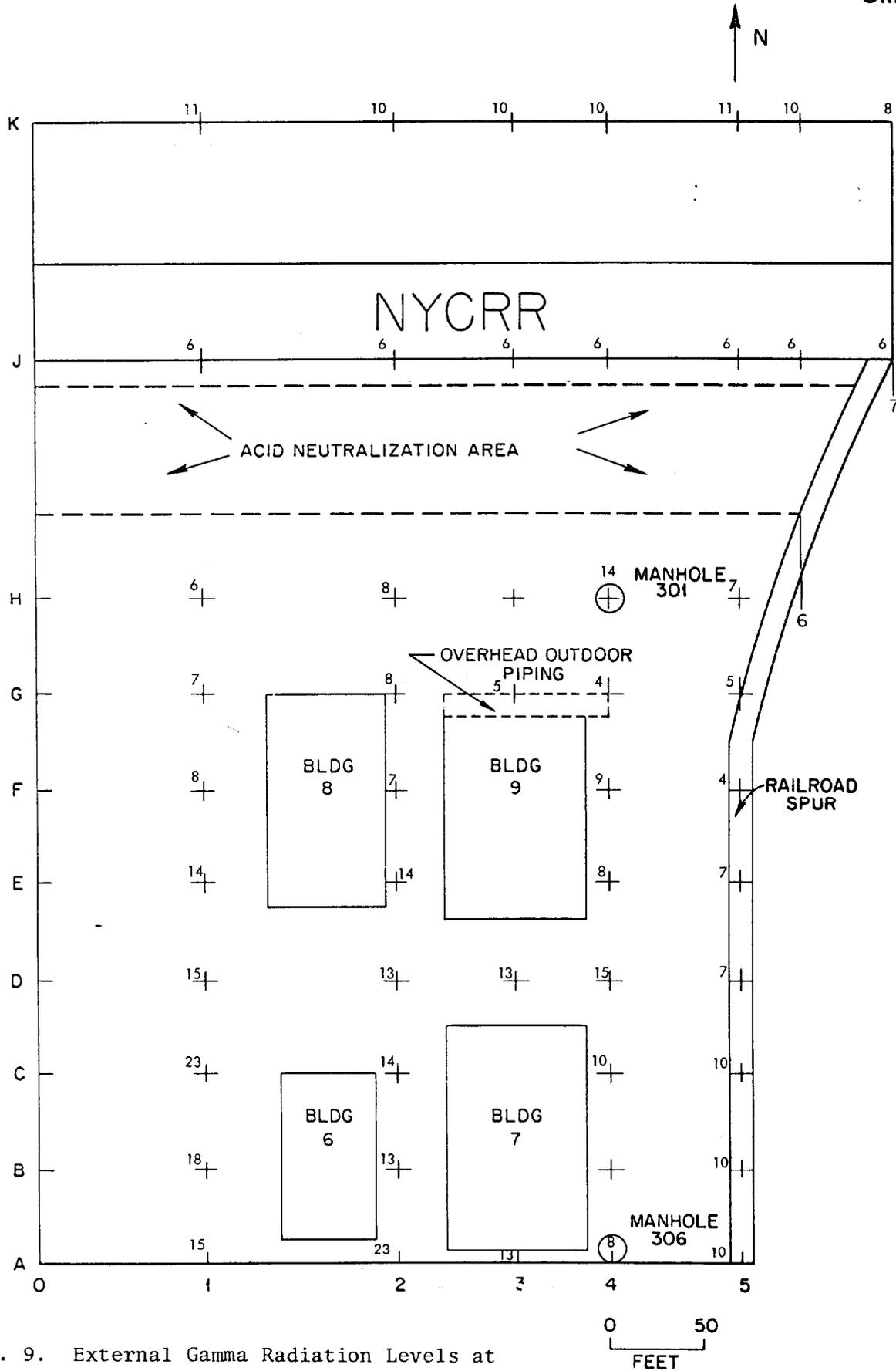
Fig. 9. External Gamma Radiation Levels at One Meter Above the Outdoor Surfaces. (Expressed in  $\mu\text{R/hr.}$ )
