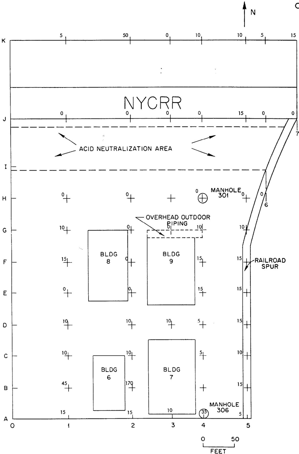
Fig. 2. Alpha Contamination Measured on Outdoor Surfaces. (Readings expressed in dpm/100 cm<sup>2</sup>.)
