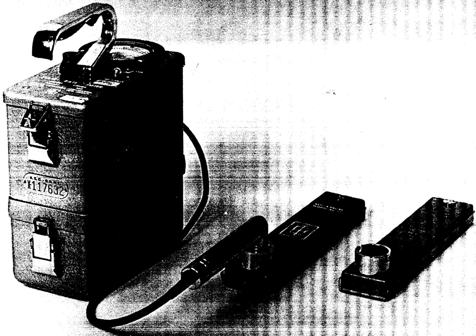
Fig. I-B. Gas-flow Proportional Alpha Survey Meter.
