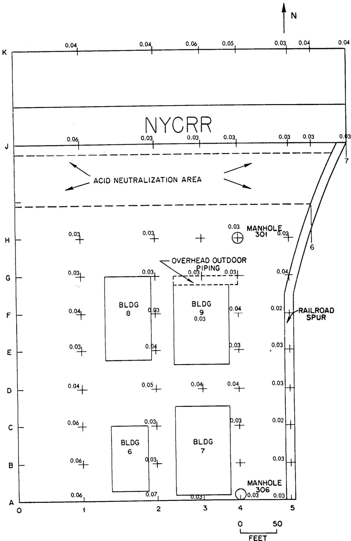
Fig. 8. Beta-Gamma Radiation Levels at One Centimeter Above the Outdoor Surfaces. (Expressed in mrad/h.)
