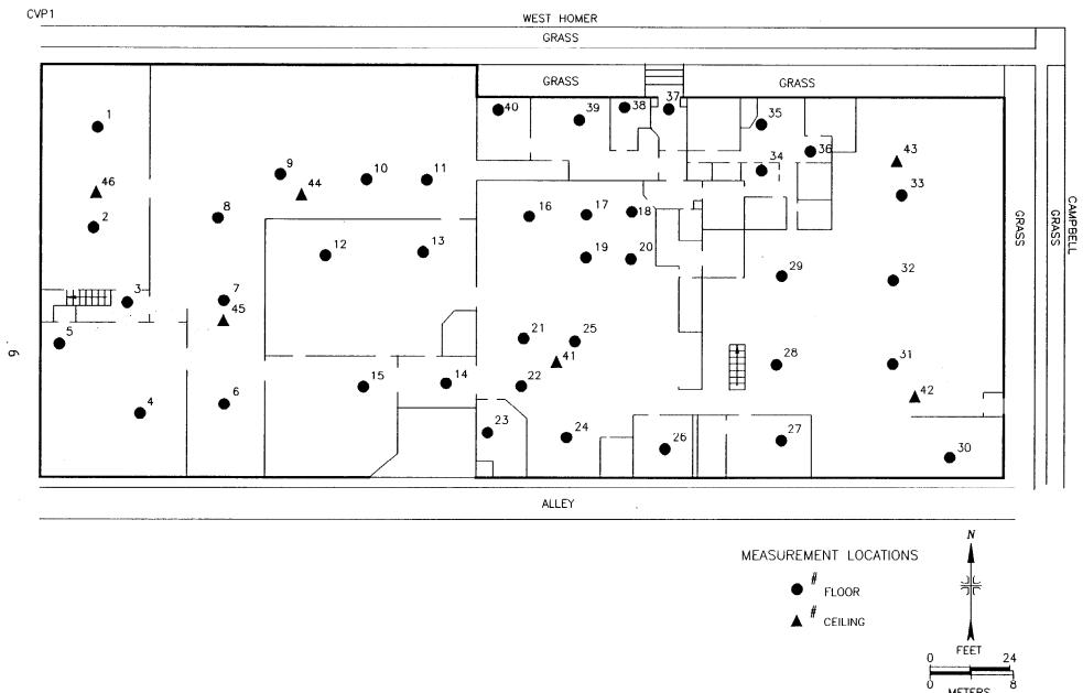
FIGURE 2: Floor Plan of 2501 West Homer Street Indicating Locations of Contamination Measurements
