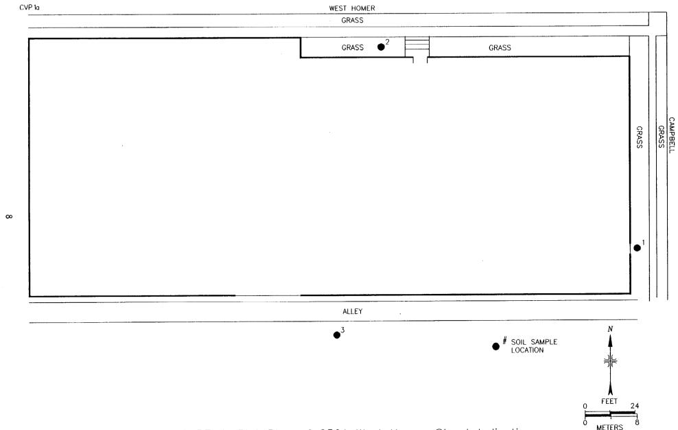
FIGURE 4: Plot Plan of 2501 West Homer Street Indicating Locations of Soil Samples
