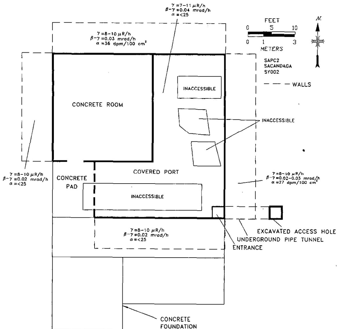
Fig. 13. Directly measured radiation levels inside the covered port of building P at the Sacandaga site.
