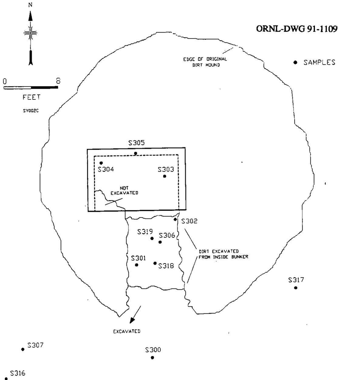
**Fig. 11.** Diagram showing the locations of soil samples collected before excavation to reveal the bunker floor and interior. The bunker and pile of soil covering it are shown as if viewed from above.
