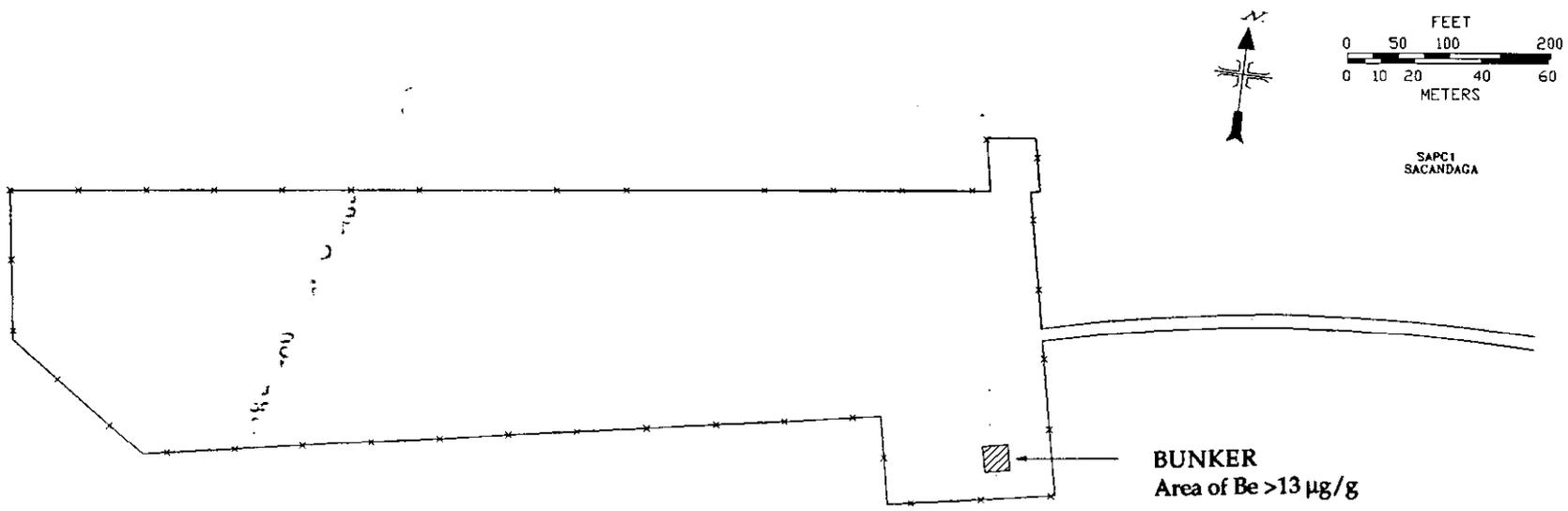
**Fig. B.1. Diagram showing the area of beryllium concentrations greater than 13 µg/g on the Sacandaga site (i.e., the concrete bunker).**
