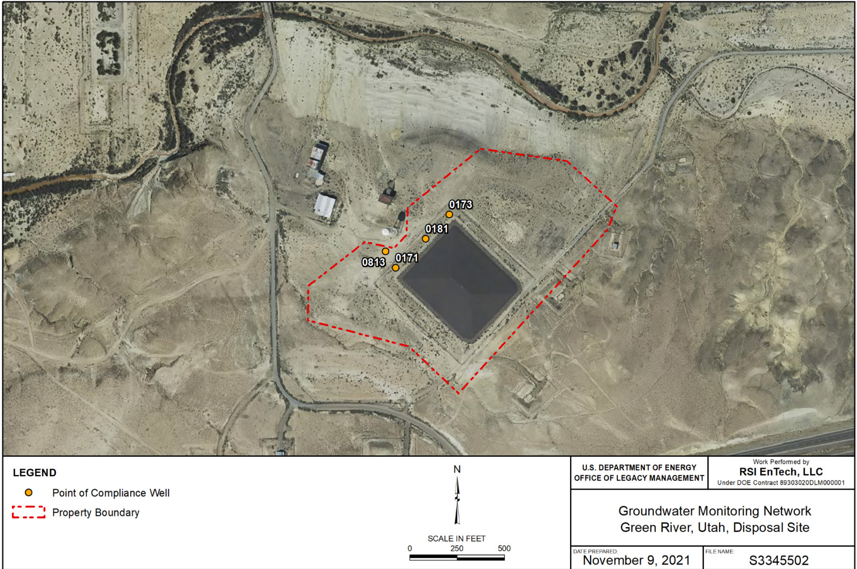
Figure 7-2. Groundwater Monitoring Network at the Green River, Utah, Disposal Site
