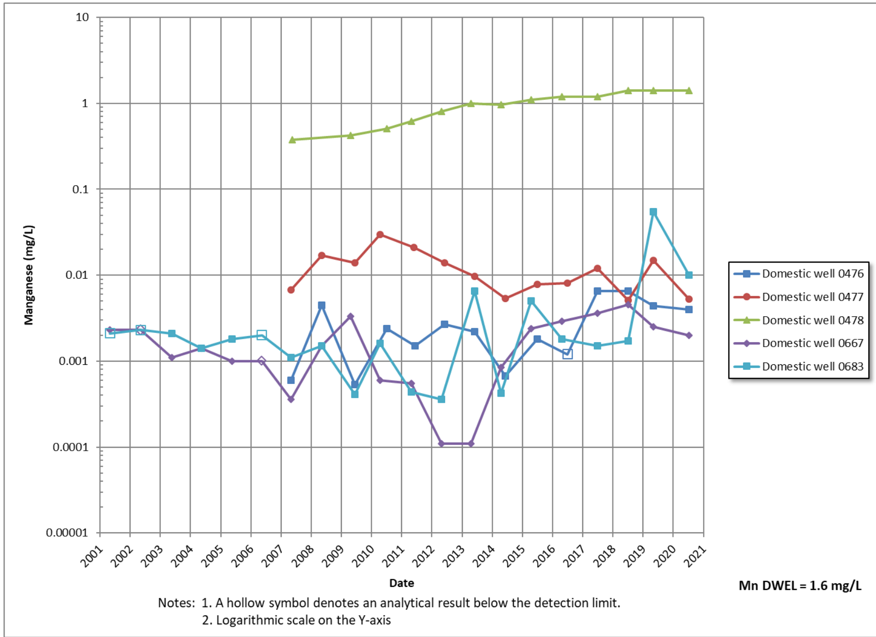
Plot 2. Manganese Concentrations in Groundwater, Domestic Wells Downgradient of the Former Mill Site (West of Gunnison River)
