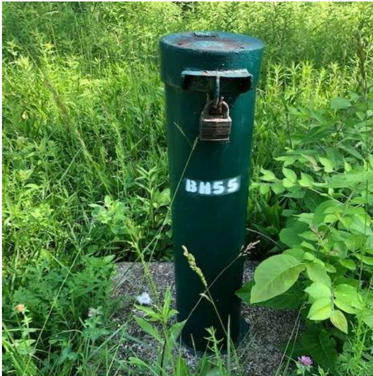
P08 - Monitoring Well BH55 at Site A
