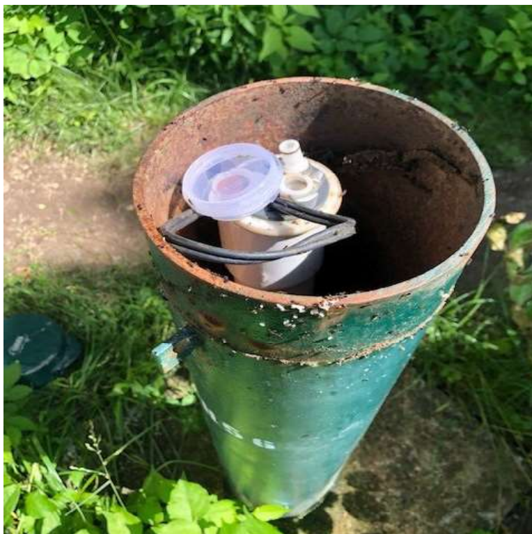
P10 – Monitoring Well BH56 at Site A, Uncapped to Depict Ant Infestation with Ant Bait Trap Resting on Top
