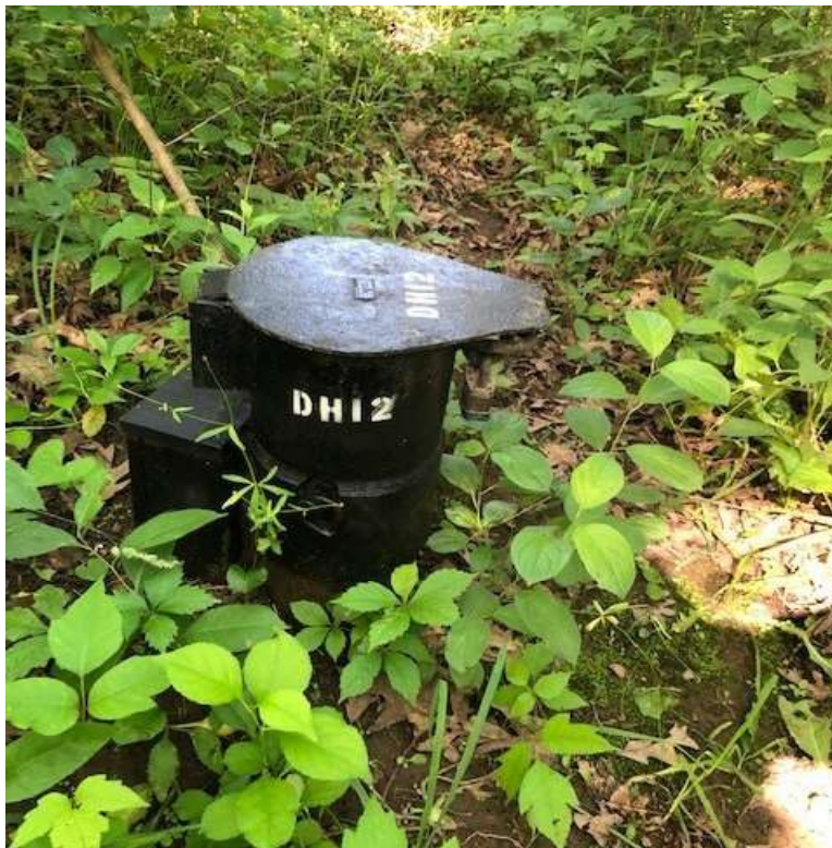
P12 - Monitoring Well DH12 at Red Gate Woods
