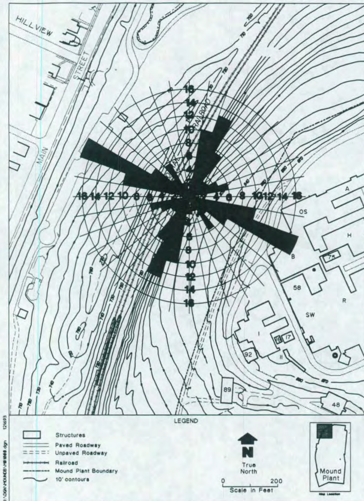
Figure 3.6. Frequency and orientation of fractures in limestones at railroad cut outcrop.
