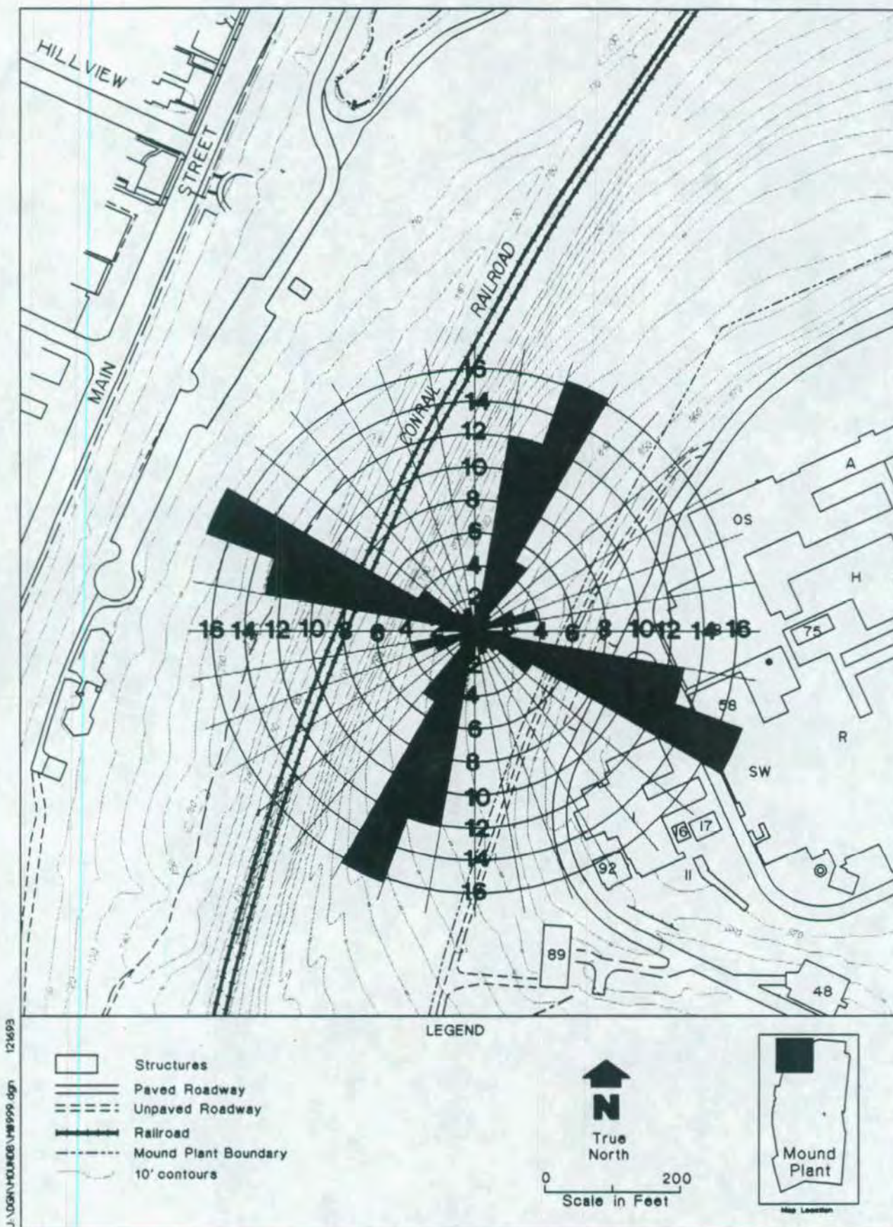
Figure 3.5 Frequency and orientation of fractures in shales at railroad cut outcrop.
