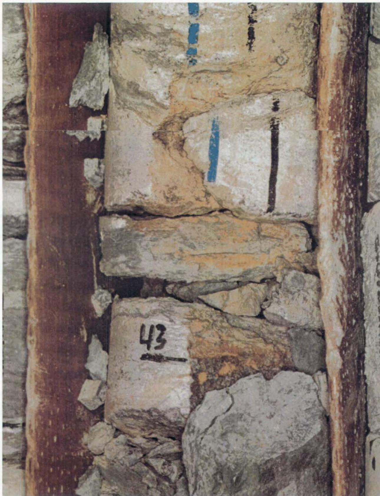
Figure 3.3. Photograph of natural fractures in core 0348 at 42-ft depth (elevation 834 ft MSL) (splice of Mound photographs #932459 and #932460).
