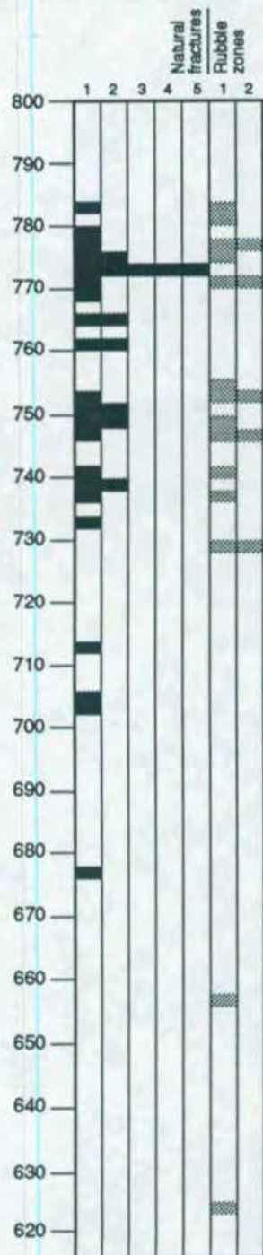
Figure 3.11. Correlation of flowmeter measurements and fracture frequency at borehole 0349.
