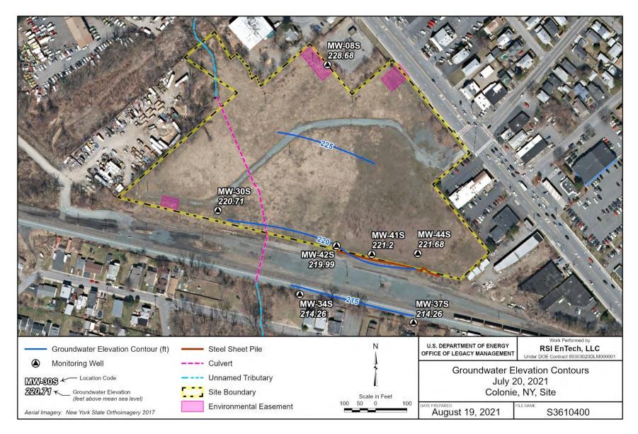
Figure 6. Groundwater Elevation Contour Map, July 2021
