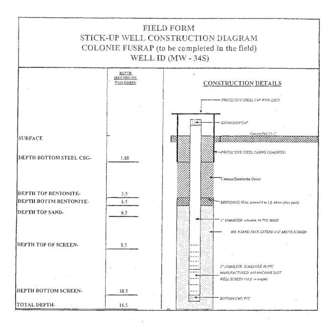
GEOLOGIST: M.Flanagan DATE INSTALLED: 12-20-01 DATE COMPLETED:12-20-01 BOREHOLE DIAMETER: 8 in. TYPE OF DRILLING:Hollow Stem Auger DRILLER/RIG: M.Marshall/Parrat Wolff
