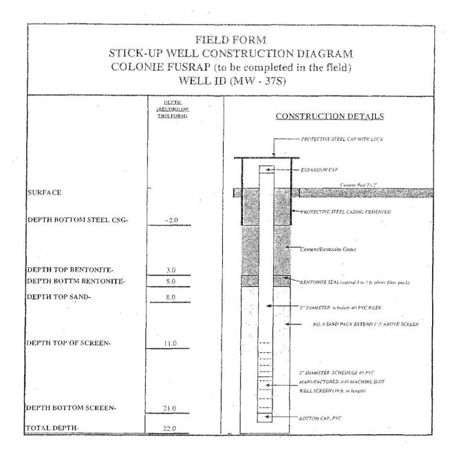
GEOLOGIST: M. Flanagan DATE INSTALLED: 1-27-02 DATE COMPLETED:1-27-02 BOREHOLE DIAMETER: 8 in. TYPE OF DRILLING:Hollow Stem Auger DRILLER/RIG: M.Marshall/Parrat Wolff
