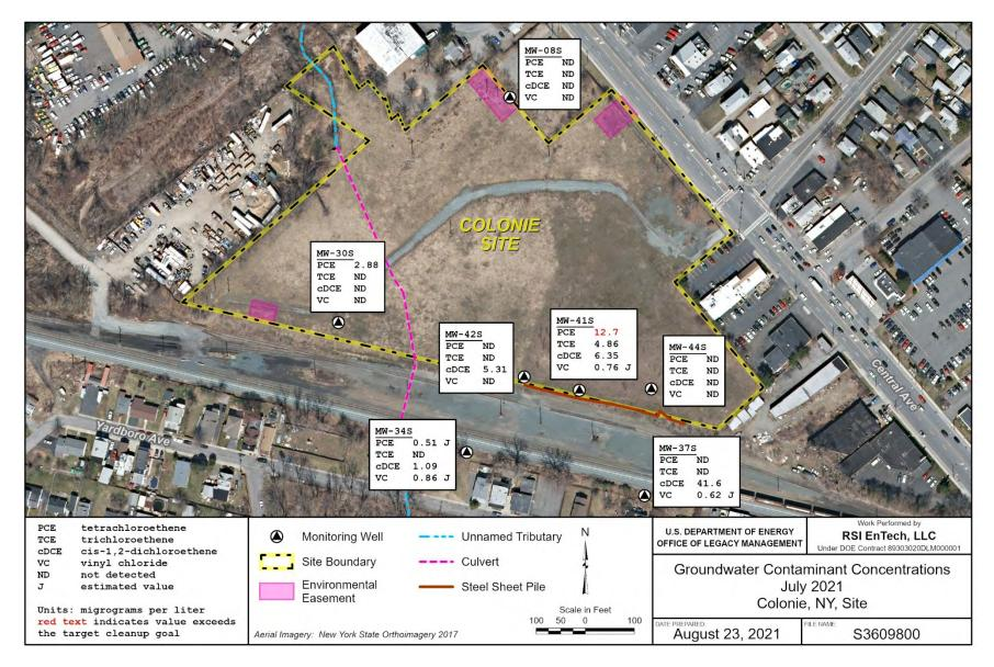
Figure 8. Monitoring Wells and VOC Concentrations
