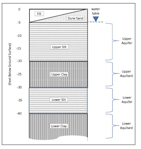
Figure 7. Generalized Cross Section
