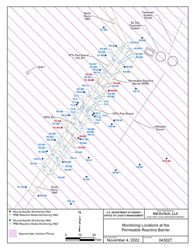
Figure 5. Monitoring Locations at the Permeable Reactive Barrier
